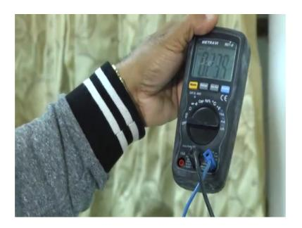
You see just it is now in the position of discharging it is the position of discharging ok. So, here initially some charge was there in capacitor. So, I will make it short to discharge it is, but it is in milli volt order. So, very small it is the milli volt order very small so, but I can make it almost 0, I can make it almost 0s are just across the capacitor I will just
