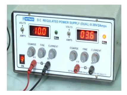
So, this is the our power supply. Basically here we will apply from here we will take the voltage for the circuit. So, here is a variable power supply we can vary the voltage. So, generally around 10 volt we will use for this experiment.
