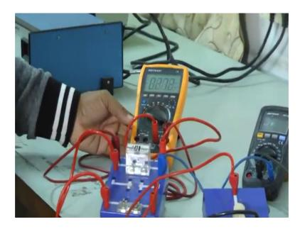
So, across the capacitor this voltmeter, so this voltmeter is connected across the capacitor right. So, here you can see this is the one end of this capacitor here ok. So, in this board basically it is internally connected. So, it is the across the capacitor this voltmeter is connected right.
