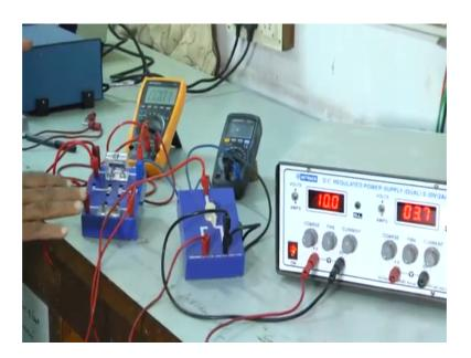
So, now, so, what we will do I will just so, it is in discharge mode ok. Now, there is no charge in the capacitor. So, that is why it is the reading is you see almost 0 right, it is a 0.3 milli volt it is current is 0 in the circuit. Now, we have to note down at t equal to 0, what is the voltage, what is the current?
