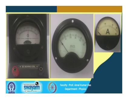
So, this just I have shown you here, this galvanometer, ammeter and voltmeter. So, it is from our lab; it is the basically from our labs. So, I think voltmeter yes it is the voltmeter, then this is the ammeter and this is the galvanometer ok.
