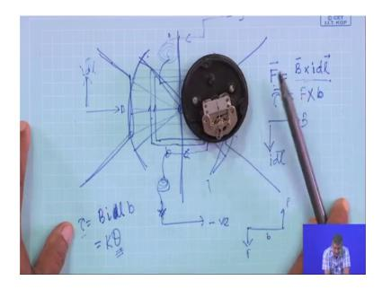
So, this torque because of this torque it is it will rotate and then you are taking basically this basically B i dl or l into B. This is basically this is the width and this is the length, with l I can write basically this dl instead of dl I can write length this is the length and this is width.
