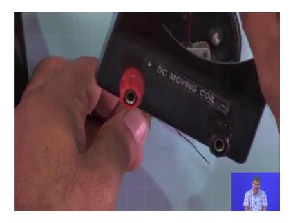
So, this externally when it is connected. So, basically these two black and red positive and negative ok; when you are putting in the circuit in a series. So, current will enters ok. So, we do not say it will enter. So, it will enter from it. So, this one is connected with the one of them is connected is connected with the basically top spring and another is connected with the bottom spring means current will enter from here, then through the top spring it will go and it will go.
