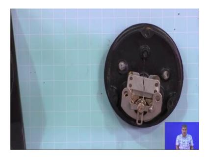
So, when current passes through the coil, then depending on the direction of the current in the coil and magnitude of the current in the coil; so this coil it is just rotate. So, this amount of rotation it will depend on the amount of the current. So, that is why this helps to know the direction of the current and amount of the current passing is passing in the circuit ok.
