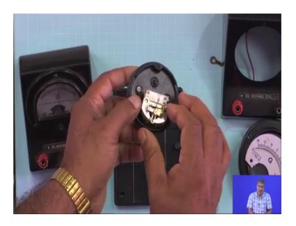
So, this is the scale, this is the indicator ok. So, this is fine what is the very small parts inside you know. So, this called moving coil galvanometer, because this principle is based on this on the moving of a coil. So, where is that coil where is that coil? I have to show you where is that coil. So, I think it is here I have to show here two parts is there you know, one is moving coil another is permanent magnets.
