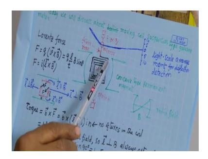
So, we will discuss about the moving coil suspension type galvanometer, moving coil suspension type galvanometer. So, this is a coil, this is a coil ok, rectangular coil. Now, this coil is suspended is hanged using a fibre rope, using a fibre rope and in between here this just we attached 1 metre.
