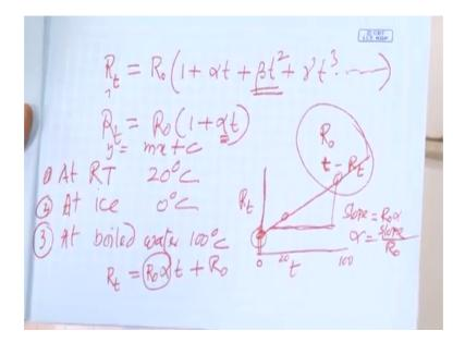
Now, I want to measure the resistance of the platinum wire right platinum thermometers ok. So, for any metal the resistance R t say at temperature t R t, so that one can write R 0 resistance at temperature 0 is 1 plus alpha t plus beta t square plus gamma t cube etcetera right. So, this is the relation between resistance and the temperature.
