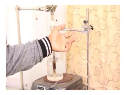
So, my task is what task is to measure the resistance. So, for so to measure the resistance to measure the resistance, I will use this bridge can you push the bridge. So, what we will do, as I told these two these two for platinum wire. So, these two we will connect in this third gap , and these two these two these two we will connect. I think this is P P. So, I think this two P P and this two C C. So, this I will connect at the gap 4 gap 4.
