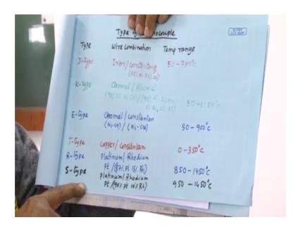
So, types of thermocouple here their different name is given you know J-type, K-type, E-type, T-type, R-type, S-type. So, this name are basically depending on the combination of the two types of wire. So, J-type thermocouple we tell when these two wires, one wire is iron and another wire is constantan ok. So, constantan means 45 percent nickel and 55 percent copper alloy ok, so constantan.
