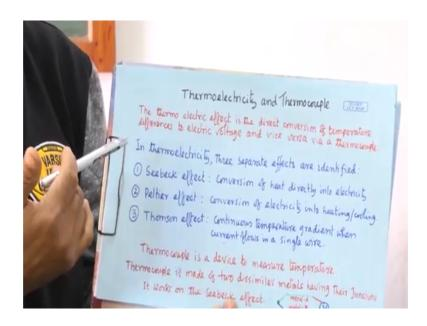
So, let us know about the theory of this experiment. So, this thermoelectricity you know this basically tell this thermoelectric effect. So, this thermoelectric effect is the direct conversion of temperature difference to electric voltage and vice versa by a thermocouple, right.
