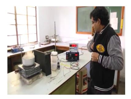
So, here this is our experimental setup for this thermo electricity and thermocouple. So, you see this is a thermocouple. So, thermocouple means two dissimilar metals, so this is one type of metal and this is another type of metal ok. So, these two metal, dissimilar metal it has junction one junction here and it has another junction here ok.
