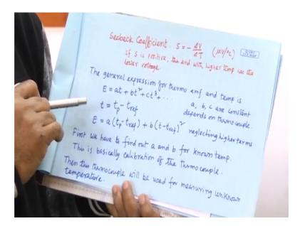
So, Seebeck effect, you know the Seebeck effect, as I told this if there is a temperature difference between the two junctions then there will be thermo emf, there will be voltage; there will be voltage in the generated in this circuit in the thermocouple. So, this Seebeck coefficient is defined as S equal to minus del V by del T ok. Del V is the voltage difference generated because of the temperature difference del T ok. So, this also this Seebeck coefficient also if it acts as a calibration.
