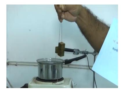
And now, it's temperature is T 2; it's temperature is t 2 and when it will so when if it is a hot body I have to make it hot see it's temperature T 2. Now if I put it in a cold body I will put in a water in a calorimeter ok. So, in calorimeter water as well as this copper container will be there and they are sealed in a in a thermal radiation so that there should not be any loss of loss of this loss of this loss of this I think I have to it's a boiling. Let me switch off this one, yes ok.
