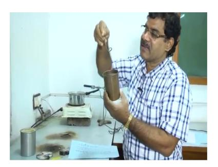
So, this is the basically calorimeter. It is the copper container calorimeter ok. So, and this is the stirrer so you get the uniform temperature, so we will use this stirrer. So with this stirrer so, we will take this weights of this ok, this is the 91.1 gram. And the specific heat of this scope of material is will be given is supplied is known. So I will multiply with this mass into this specific heat of this copper.
