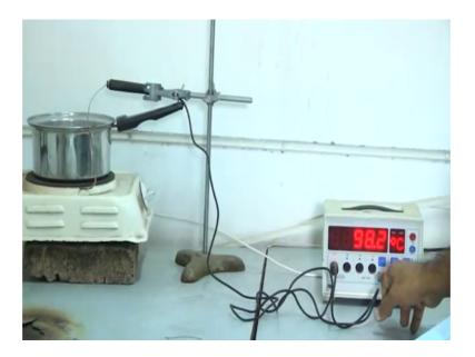
So, this thermocouple is there, so this is the here we are getting the reading of the temperature from this thermocouple ah. So, this is the I think this is the yes; this thermometer is a thermocouple type. So, there it's a here this reading of this water temperature of this water is 97.8 is decreasing, so I think I will switch on this 1 now; so ah. So, this type of metal already another metal i put it here, you see here I think it's a aluminum ok. So yeah this is the aluminum metal ok.
