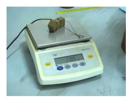
So, we will measure the mass of this hot body. So, before give me putting there we I should take mass ok. So, it is showing this 178.5 gram this one. So, we will do this experiment for 3 metal. So one is aluminium there one is this is iron basically ok. It is a iron this metal is iron and this material is brass basically, here another sets of material I have taken ok. So, this is the copper zinc alloy so it's brass basically ok.
