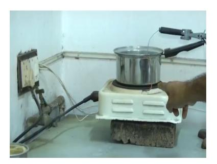
So, here you see water is boiled just I kept it in boiled boiling condition, because then we will lose time we will not lose time. So, this is a thermocouple is put in the; so this is the heater on this heater I put water in a container I took water this power is given from there
