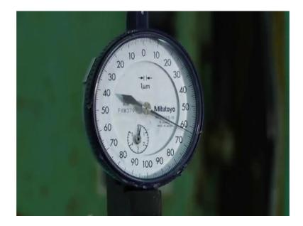
So, now you see here this one setup, where this one is called micrometer and this rod when rod will be expanded. So, this arrangement is done in such a way the how much it is expanded. So, this from this reading we can tell that is the expansion of the rod and now why rod will expand. So, if we increase the temperature of the rod, then it will expand. How much it is expanded, so that reading we have to take that will be taken using this micrometer.
