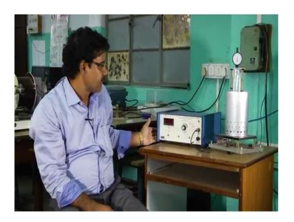
So, this is the experimental setup for measuring the thermal expansion of a metal rod ok.
