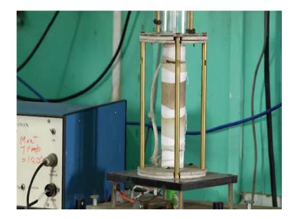
Then actually here this thermal insulators asbestos it is called I think a ceramic kind of things is used. So, this rod is basically inside of this ceramic cylinder. So, now surrounding the rod, there is a coil where there is a coil heating coil basically.
