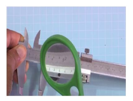
Here you see, it is coincide with the main scale division yeah. So, 27 one can take ok. So, 27 into this vernier constant so that that will be the vernier reading and so, main scale reading plus this vernier reading. So, that will be the final reading minus initial reading, it is a 0, because zero error is nil so that would be the depth ok.
