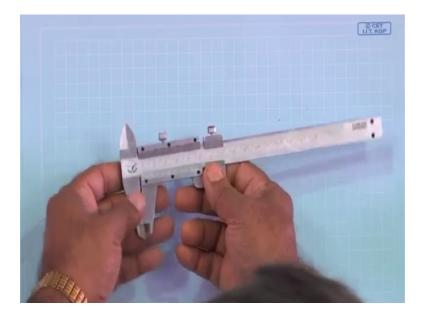
So, it has zero error it has it has no zero error as I showed you, it has no zero error right it has no zero error it has no zero error, it has no zero error ok. So, this is used for as I told this inner measuring jaw. So now, what is the use of that? So now, if I ask you what is the internal diameter of the cylinder?
