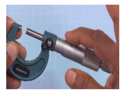
And this is called this here this basically, 2 scales are there one is circular scale, this circular scale ok. So, in this case, it is the it is 0, 1, 2, 3. So, up to in circular scale, this is total 50 divisions are there and then this is called these are main linear scale circular scale and linear scale. So, in linear scale this is the divisions are in millimeter, and so this is the circular scale ok.
