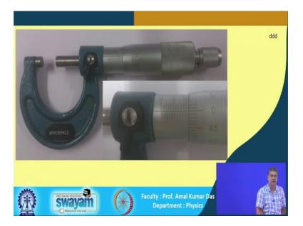
The next I will go for this screw gauge. So, another tools for measuring the length ok. So, that is the screw gauge.
