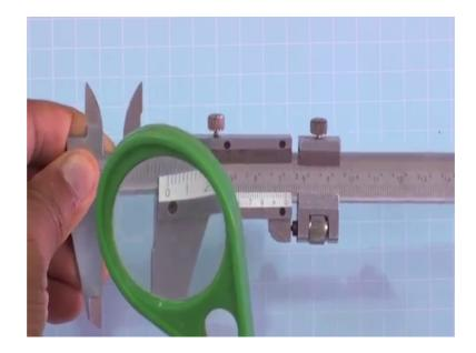
So, it is not difficult to find out here is you can I can see 1, 2 centimeter and then 2 then 1, 2, 3. So, 2.3 centimeters and then after that this 0 vernier 0 and then I have to see how many division coincide with it. So, it is around 25 around 5 that there 5 means 35 division or 26 division or 27 division almost, it is coincide with the 27 division.
