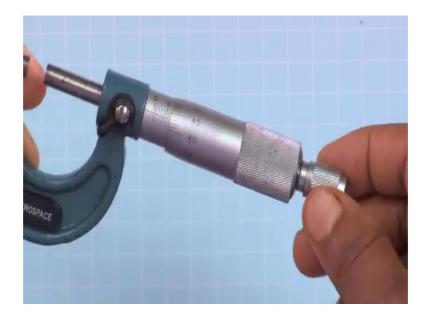
And this called ratchet, this is called ratchet ok. So, this helps to know that when you are putting anybody you need to measure the thickness are diameters of in wire. So, we put the things in your (Refer Time: 07:20) So, how long you should place? So, after just touching it, if you just use this one then it will just give a sound; that means, the end your you can stop this pressing ok; that means, this is the right position for this thickness of diameter and then you should take reading ok.
