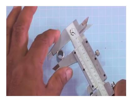
So, this is for measuring for external diameter this will be used for internal diameters ok. Now, if I ask you what is the depth of the cylinder? Then how we will measure, the depth of the cylinder?
