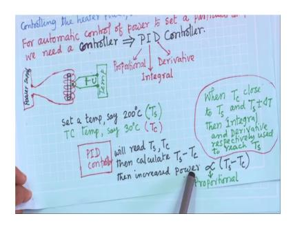
It is a basically controller, it can calculate. So, electronic circuits are there ok. So, it will calculate difference between these Ts and Tc, then increase power proportionally to the difference of this temperature. Initially it will increase power which is proportional to the difference of temperature because initially there will be big temperature difference. So, it increase proportionally. So, that is all this proportional PID P that proportional that is coming.
