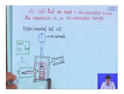
So, then next another parameter is there is no working formula that is del L that is del L. So, del L tells that we did not show this expansion and we need to measure this expansion, we need a micrometer since this expansion using a micrometer range. So, then we tell this so micrometer which will read the expansion in the range of micrometer ok.
