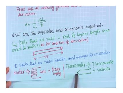
Then t in derivation; t is there in working formula. So, t tells that t means temperature right we have to change the temperature of the sample of the specimen right. So, how to change the temperature? So, we need heater as well as we have to read the temperature of the specimen ok. So, we need thermometer ok. So, heater is nothing, but so, this we can take a coil and we will insert this rod into this coil ok. So, heater is basically is coil and we need power supply ok.
