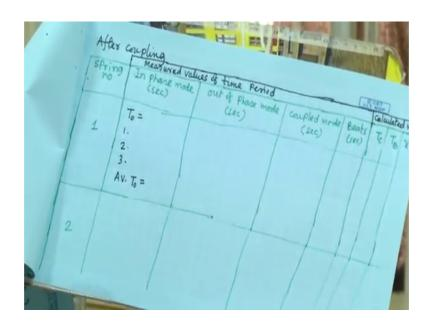
So, now we should go for after coupling, so I will just show for spring 1 for spring 2 you can repeat the experiment what I have to find out actually I have to find out T 0 and T 1 right this there. So, T 0 what is this in phase mode in phase mode I can find out the frequency that is the T 0 and out of phase mode out of phase mode. So, what about the frequency I will find out, so that is the T 1 so that is what I will find out.
