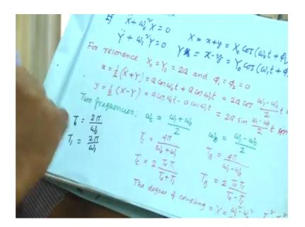
So, here that is why omega c we have written equal to omega 1 plus omega 0 by 2 omega B we have written that is equal to beat frequency that is equal to omega 1 minus omega 0 divided by 2 ok. So, omega you can convert to in terms of T time (Refer Time: 22:09). So, that is why T0 and T1 that here I have shown the relation.
