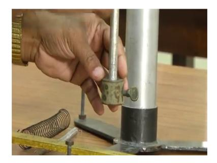
So, pendulum for simple pendulum you know this there is a mass is hanged with a jelly thread, but here hanged with a light rod; it is a light rod and this mass is heavy compared to this rod, so this is see this a simple pendulum. So, we can find out the time period of a simple pendulum how to find out that we try, just I will displace it; I will displace it and I will I just use stopwatch.
