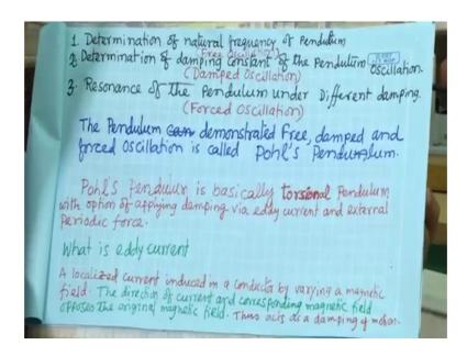
So, let us come to the to study this oscillation, we will use this Pohl's Pohl pendulum as I told, so what is Pohl pendulum what is Pohl pendulum. So, how we are getting, how we are applying, how we are applying damping, how we are applying external force in this in this setup. So, Pohl's pendulum is basically the torsional pendulum with option of applying damping via eddy current and external periodic force ok.
