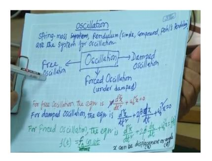
We are in first year laboratory of physics department of IIT, Kharagpur. So, today I will demonstrate one experiment that is basically oscillation and we will start with the oscillation. So, oscillation you know this spring mass system oscillate, then pendulum, simple pendulum, compound pendulum oscillate right.
