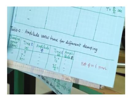
So, this damping current, for a particular current, so I will take this amplitude at 0, t equal to 0, at t equal to 0, at T, 2 T, 3 T, I will note down here, then other side as I told this at time T by 2, 3 T by 2 we have to note down, then we can plot phi versus time graph ok.
