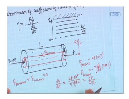
If we equate this two, so you can basically write d v by d r equal to, so minus sign will go this here this pressure. So, it take in opposite side d v by d r equal to del P pi r square divided by eta 2 pi r L right. So, this basically you are getting delta P pi pi will go r this will go by 2 eta L; 2 eta L. So, here d v by d r equal to del P by 2 eta L.
