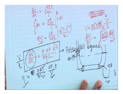
So, d v by d r equal to delta P by 2 eta L. So, del P file wherever the pressure we are applying between these two end of the capillary tube L also length is known we will measure the length. Now what is d v d r d v by d r how to measure is a directly we
