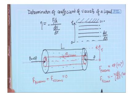
So, basically ours experiment is determination of coefficient of viscosity coefficient of viscosity of a liquid. So, basically in a laboratory we will measure the viscosity of water. So, so this definition of viscosity coefficient of viscosity say it is eta it is a equal to
