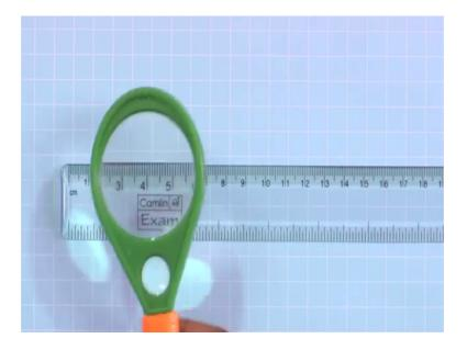
So, we have meter scale and theirs this least count is millimeters because between this 1 and 2 say between 1 and 2 how many lines are there? This you can count it is 10 lines are
