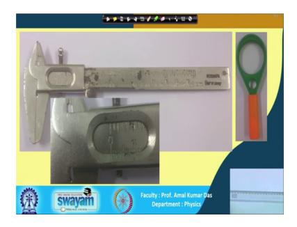
So, next first we will discuss about the slide calipers; that is actually in class 11 student do this experiment. But I will then just discuss once more because in whole life for any experiment most of the experiment we need this instrument, and we should have clear idea about this instrument how to use and what is the significance of this instrument.
