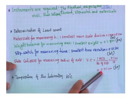
So, basically this flywheel we have seen the flywheel and then weight or mass, then balance to measure the mass or here we have been measure weight balance or anyway simply balance. Then mass, then we need slide callipers, thread, stopwatch and meter scale ok. So, these are the instruments we required for this experiment.
