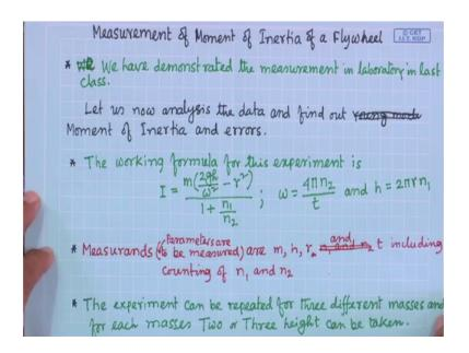
So, in laboratory you have seen the instrument and how to perform the experiment that we have discuss. So, let us now analysis the data and find out moment of inertia and errors on the measurement. So, the working formula for this experiment is I equal to m 2 g h by omega square minus r square divided by 1 plus n 1 by n 2.
