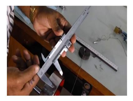
So, we will use as usual this slide calipers ok. So, slide calipers we will use to measure this diameters or radius. So, you know already I have discussed about this slide calipers, then how to use it, how to take reading right. So, slide calipers just we will use here this just yes first we have to take this whether is there any 0 error and then we will take this reading for this for this place.
