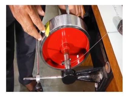
So, this is the basically this is the flywheel. So, I think yes this the flywheel. So, it has we can see this it has axis this flywheel, this it rotate about this axis right.
