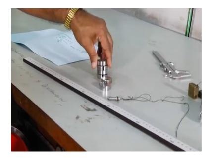
So, we have this mass of 50, it is a 50 gram. So, we have 50 gram mass. So, you put 2 3 4 mass together hang with this thread and for different mass also. So, one can do this experiment repeat the experiment for 2-3 mass also. So, for 2-3 height and or 2 3 mass
