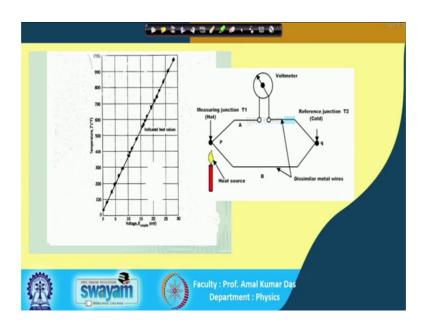
So, thermo couple basically what is thermocouple? This two dissimilar metal if we make two dissimilar metal if we make junction. So, this is may this is the wire of wire A and this wire B. So, it is a wire is made of some metal metal. So, may be copper and this where B is made of some other material. So, this it has to be dissimilar material. So, if you take this two dissimilar material and then this if you make junction here, ok. So, this
