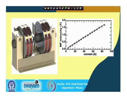
And another if you want is not magnetic field thermometer that this magnet electromagnet. So, how to again, there are two coils, there are two coils placed and this pole pieces are there. Now, if you first find through these coils and then there will be magnetic field between this two pole pieces again. So, what is the relation between the current and magnetic field?
