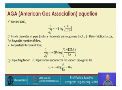
Now, for the American Gas, Association that is AGA, there is another equation, for the, this Reynolds number and this is given in terms of the, this, friction factor and this, we know that this is, for a rough pipe, and here we have For partially turbulent flow we have this particular expression, and, mind it that all these things are in the FPS units ok, then that is how this particular, quotient is 1.412 or 3.7. They are coming due to the particular, this, this expression of this unit system.
