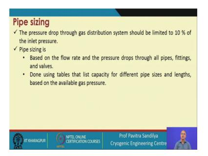
Now, after knowing these, pressure drops we go to the Pipe sizing and this Pipe sizing what we mean that we have to decide that what kind of diameters, of the pipeline to choose, for a given length. So, this pressure drop to the, gas distribution system should be immediately about 10 percent of the inlet pressure. So, this is a kind of a thumb rule we follow to design the pipe, pipe size to design the pipelines.
