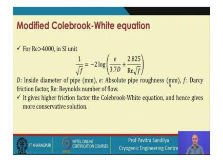
And in this first, we shall see the Colebrook-White expression and in this we find that in the FPS system for a large number more than 4000 is given by this particular expression. So, in this we find that the diameter and the, roughness factor is given in terms of inches and. So, and this particular expression is we find that this first term is signifying the roughness effect and the second term is signifying the Reynolds number effect.
