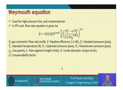
Now, another popular method is Weymouth equation and this Weymouth equation is used for high pressure pipelines and for example, also we may use used for compressed air. So, in this case for FPS system of units we find this is the expression for the volumetric flow rate by the Panhandle, expression and here again we find the similar the equation looks, similar to the Panhandle A or Panhandles B, only thing is this here the values of the coefficients have been changed.
