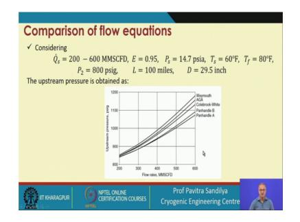
Now, in a similar manner what we can see, that we can also find out the other way; that means, now in this case we are given the, outlet pressure, and from that we are, we want to know what is the inlet pressure. So, in this again we find that so, this is the, range of the flow rates and now we are putting in terms of flow rate and length is taken to be a constant and this is some other diameter of the pipeline, and again the pipeline efficiency is taken to be 95 percent.
