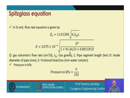
And the similar expression is given for the SI units again you see that this particular value and these coefficient values have changed for the, different types of units and. So, has the value of this particular a coefficient.
