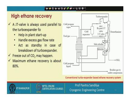
Now, a JT valve is always used parallel to the turbo expander here we are using parallely to turbo expander JT valve why to help in plant start up handle excess gas flow rate and act, act as standby in case of turbo expander.
