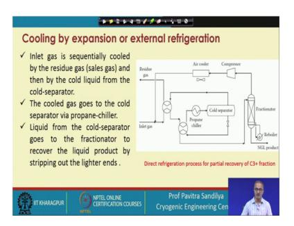
Now, here we have a typical flow chart for the expansion or external refrigeration. Here we find the inlet gas is sequentially cooled by the residue gas or the sales gas and then by the cold liquid from the cold separator. So, what we find? Here we have the inlet stream. So, here the inlet stream is first been cooled by these residue gas which is obtained from the cold separator.
