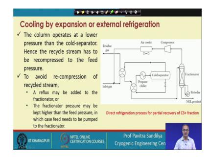
The column operates at a lower pressure than the cold separator. Hence recycle stream has to be recompressed to feed the feed pressure. What it means that because this particular thing fractionators has a lower pressure than the feed pressure is the cold separator.
