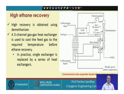
Now high recovery is obtained using demethanizer as we have seen again this is the conventional turbo expander based ethane recovery system. So, here we are has in demethanizer this is from where we are getting this high ethane recovery.
