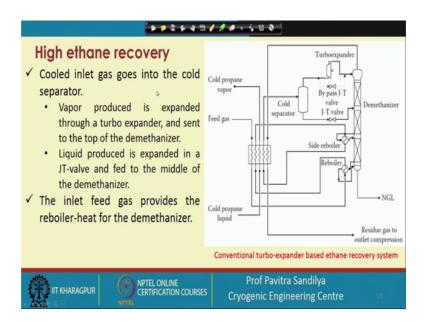
Now you can see here that the cold inlet gas goes to the cold separator. Now you see that how the cooling is getting done that the feed gas is coming through some heat exchanger. And here this heat of the feed gas is also used in the reboiler to boil up the liquid in the demethanizer. So, this is this that means, this heat is used as boiler. So, that is why this feed is get is getting cooled and it is colder than the initial feed gas.
