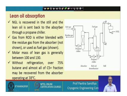
NGL is recovered in the still and the lean oil is sent back to the absorber through a propane chiller. Now here in this is the still. So, here we see that in the still what we are doing that we are getting this rich oil from the bottom of the still and it is being sent back to the absorber through this propane chiller over here.
