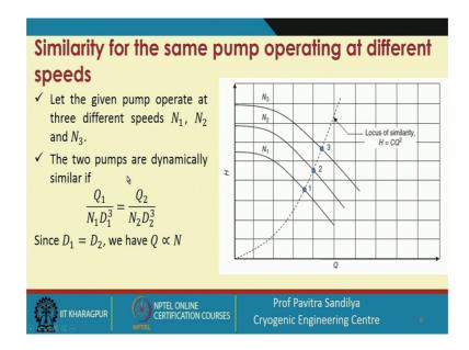
So, here we have the things that here we have first you see that similarity of the same pump operating at different speeds. So, let us see that N 1 N 2 N 3 are the various types of speeds of the pump.
