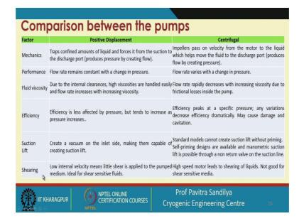
And here is a small comparison between the different types of pump this is a positive displacement pump and the centrifugal pumps. And their differences are on various basis like the on their mechanisms, their performance, then fluid viscosity they can handle the efficiency the suction lift and the shearing.
