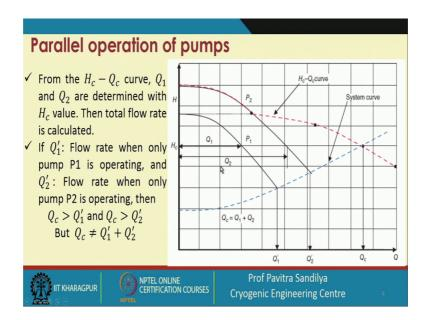
Now, here we see the H c curve that H c Q c is the overall head versus flow rate curves. So, here we are plotting all these. So, we can see that here we have this curves this particular thing this red one which you can see this is the H c Q c curve and whereas, this black one this is for pump one and this black one is for pump two. So, from these we can find out the flow rate which you need and here this blue dotted one is showing the overall power resistance curve.
