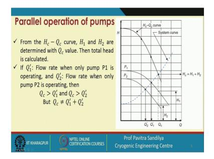
Now, here again as we saw for the parallel connection again we have the overall H c Q c curve over here. And this blue line is the overall system curve and wherever they are intersecting from this we can read out the total flow rate here, and this is the total head generated by the pumps, this is H 1 plus H 2 on the other end.
