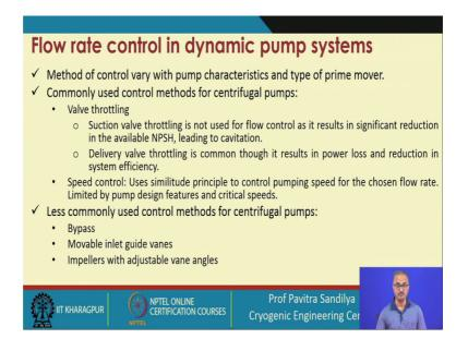
Next issue comes whenever we are going for the pump operation how to control the flow rate. Now the control the flow rate we have various methods and this method of control will vary with the pump characteristics and the type of the prime mover that is the rotor ok.
