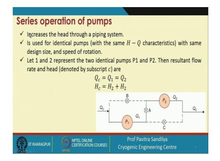
Now here we have the series operation of the pumps. So, let us first see that how these two pumps are arranged. So, this is the total flow rate which is coming and this total flow rate is going fully into this pump one and then it is going to the pump two and before it is coming out of this
