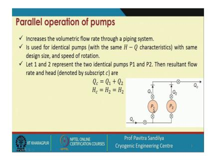
Now here we first see the parallel operation of pumps and why do we need to make the two parallel connections; now you see here that we have two pumps P 1 and P 2 and parallel means. That we are getting from some particular source is same this flow rate and which is being distributed between these two pumps they are getting parallel and then from the outside these two pumps are producing this flow Q 1 and Q 2 and ultimately these two things are coming together and going outside.
