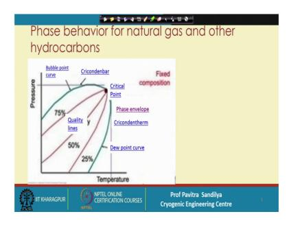
Now, first let us come to the phase behavior of the natural gas. Here, we have drawn a typical diagram with respect to pressure and temperatures. This diagram is not unique, in the sense that depending on the type of natural gas, we will be having different types of this phased diagram, though the overall features which are shown here and discussed will be the same.
