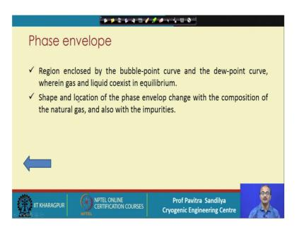
Now first let us see the phase envelope. Now, what is phase envelope? Phase envelope is the region that is enclosed by the bubble point curve and the dew point curve and this bubble point curve and dew point curve; as we learnt earlier are the ones which dictate the pressure and temperature at which the liquid phase may go to vapor phase or the vapor phase may vapor phase will go to the liquid phase.
