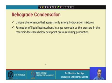
For natural gas and petroleum this is for both petroleum reservoirs as well as well as from natural gas because we learnt earlier that natural gas comes out from the reservoirs which may also contain the petroleum. So, there is a very interesting phenomena that is called the retrograde condensation and what is this retrograde condensation and why it is called. So, let us see.
