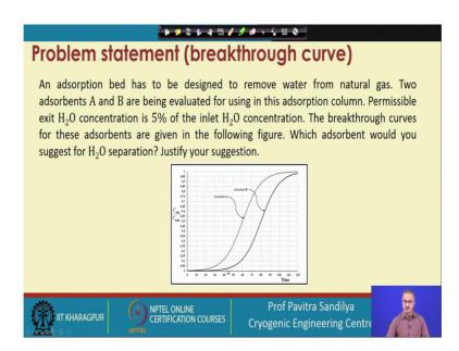
Next, we come to a breakthrough. Now, we learned about breakthrough. Their breakthrough indicates that, when a particular adsorption bed will be taken has to be taken for regeneration.
