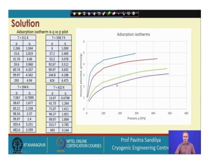
So, first we shall talk about the temperature of 311 K. And here we have the plotting; on the x axis we are plotting the pressure and you have to choose appropriately the skill and on the y axis we are plotting the adsorbate loading in terms of the millimol per gram.
