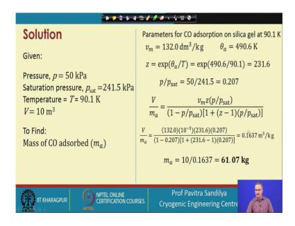
And now, we shall be using these from this vm and theta a, if we find the value of z which is needed for the BET isotherm. And when this is the BET isotherm here, and here we find the ratio of p by p set as 0.27 and then we keep on plugging in the values of the various parameters in this equation.
