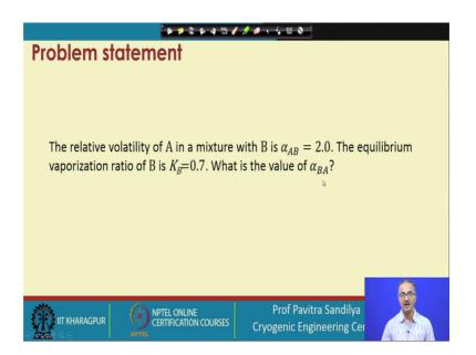
Now, first we shall see this problem, this problem states that we have the relative volatility of a component A in a mixture of B and we are given alpha A B as 2, this value shows that A is more volatile than B that because it is this alpha A B is more than 1, the equilibrium ratio A of B is KB is given as 0.7; that means, KB is the equilibrium vaporization ratio or the volatility. The volatility of B is 0.7 and we have been asked to figure out the value of alpha B A.
