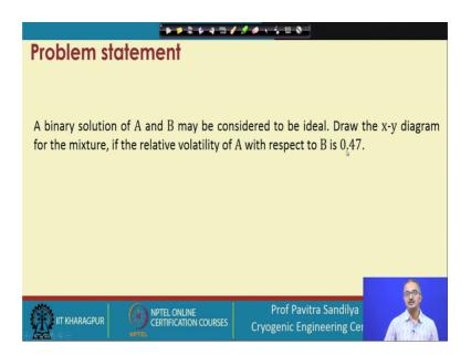
Now, next problem statement comes like this here we are trying to use the knowledge of the relative volatility to generate the composition diagram of a vapor liquid equilibrium system. Here, we are given a binary system A and B which is taken to be ideal and we have to draw the x y that is the x is the mole fraction in the liquid and y is the mole fraction in the vapor and for the given value of the relative volatility in this case we find that it is 0.47, it means the A is less volatile than B.
