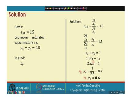
So, in this case what we do we go by this thing that alpha A B is 1.5 and the vapor mixture is equimolar; equimolar means the mole fraction of A is equal to mole fraction of B and because the summation of the mole fractions is always 1. So, we divide 1 by 2 and we get the mole fractions of A and B as 0.5 and what we have to find out; we have to find out the mole fraction of B in the liquid phase for solution of this problem.
