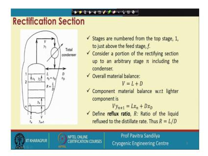
Here we first consider the rectification section or the enriching section here we what we do, that we number the stages from top to bottom as 1 2 up to small n and this well this particular section comprises of the stage just above the feed stage. So, here; that means, this particular section will move just above the feed stage.
