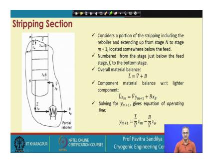
Now, then we go to the stripping section. In the stripping section what we find that we are now considering the stages which are below the feed stage against as we did for the rectifying section. In this case we are having the similar nomenclature the only difference is this in this case we are putting the liquid flow rate with a over bar.
