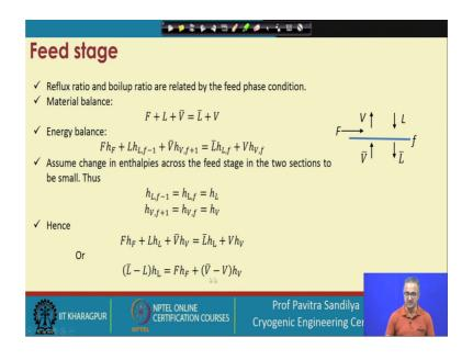
So, we find the slope of this particular line is this V B plus 1 by V B and if we extend this particular line downward, we will find the intercept will be minus 1 by V B. Now we go to the feed stage now what is feed stage? Feed stage basically correlates the boil of ratio and the reflux ratio and we will see how it is done.
