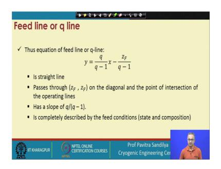
And then what we do, we write the this equation this is the feed line or q line this gives us the locus of the intersection of the operating lines of the stripping section and the rectifying section.
