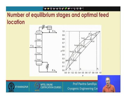
And once we have done that then what we can do simply do that, we can start making these stages as I explained earlier I can keep making these staircases to get the number of stages in the total column. Only thing one has to remember that when I am above the feed, I will be using the operating line for the rectifying section and as soon as we cross the feed we shall be using the operating line for the stripping section, and that is how we can construct the staircases from the top to the bottom.
