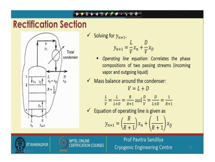
So, with this definition of reflux ratio what we do we are reducing if the this particular equation as yn plus 1 L by V xn plus D by V into x D.
