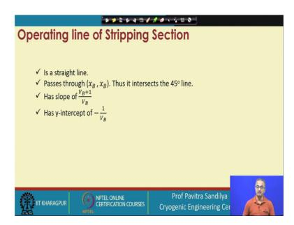
Now we find that these operating line equations is a straight line as long as the boil of ratio is constant, and when we put xm equal to x B we find ym plus 1 is also equal to x B; that means, this operating line passes through x B x B so, that one end of the operating line is on the 45 degree line and this has a slope of V B plus 1 by V B and then y intercept of minus 1 by V B; that means, it will be below the 0 x axis.
