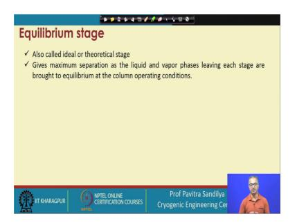
So, now, next to come to the equilibrium stage and equilibrium stage is also called ideal or theoretical stage, and the name suggests that it gives the maximum separation between the liquid and the vapor because the liquid and vapor are so intimately contacted for a long enough time. So, that these 2 phases come to equilibrium and that that will give us the maximum possible separation under the given condition in the column, that is the pressure and temperature.
