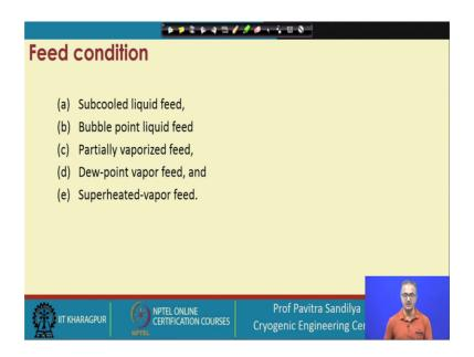
Now, there can be various types of feed possible sub cooled liquid bubble point and liquid feed, and partially vaporized feed dew point feed.
