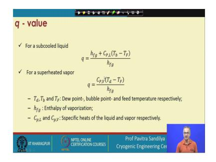
Now, with this we find that this is the way we can also find the value of the for a sub cooled liquid that achieves is the enthalpy vaporization, and the sensible heat to convert the feed to the bubble point and is fg, and for the superheated vapor we simply subtract the sensible heat from the dew point from the dew point to the feed point feed temperature.
