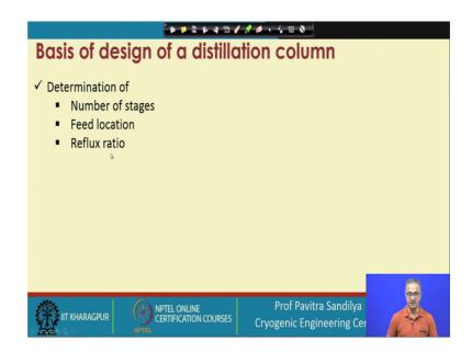
So, the basis of the design for these columns are that we determine the number of stages the location of the feed to the column and the reflux ratio.
