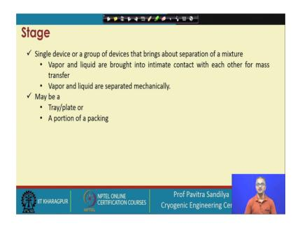
Now, first let us see what is a stage. Now stage is a single device or a group of devices, that brings about some separation to the mixture and in a stage what happens? First the vapor and liquid are brought into intimate contact, and then they are mechanically separated.
