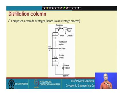
And here we find that the column is taken to be comprising various stages that, earlier we found at the total column was given in terms of the trays or the packing, but now we are putting the column in terms of stages.
