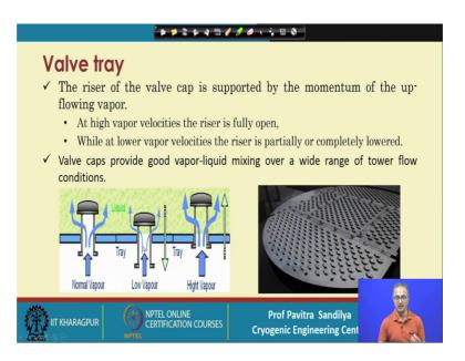
The improvement comes in the way of reducing the pressure drop across the valve. So, what we find that the valve cap is again similar to that, but there is a simpler construction this, this is the valve and what happens this valve just moves up and down this thing along with this particular riser.
