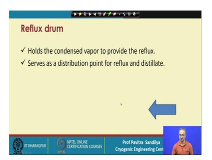
And what is job is it holds the condensed vapor to provide the reflux and serves as a distribution point; that means, we are keeping the condensed vapor in the reflux drum and we are adjusting the amount of reflux to be given to the column and so, the distillate amount will also will be changing.
