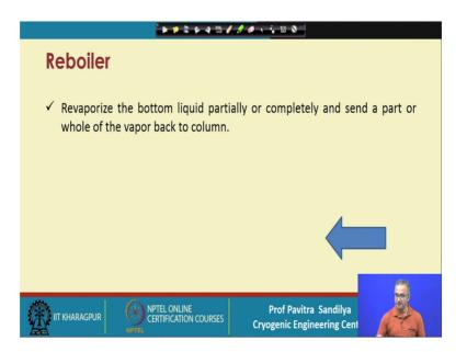
The reboiler; what it does that it revaporizes the bottom liquid either partially or completely and send a part of the whole vapor to the column and then what we find that from the reboiler, we are getting the bottom product. So, this is a typical configuration of a distillation column variations may be found as per the different types of separations by distillation in different applications.
