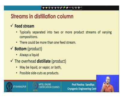
Now, the basic streams which are needed in the typical distillation column are a feed stream the feed stream will be having 2 or more than 2 components and which will be
