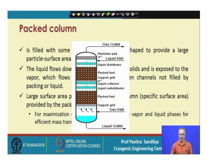
So, here we find a typical packed column, here we find that we have the packings at both the rectifying section and the stripping section and here we have some support grid to support the packing. So, to make them stay in place and then we have some liquid distributor.
