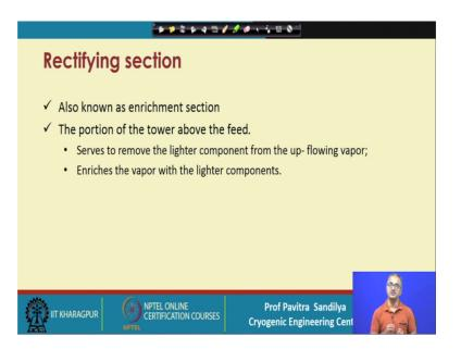
This rectifying section is also known as enrichment section and this is the portion above the feed and it serves to remove the lighter component from the up flowing vapor; that means, what will happen the lighter components from the liquid phase will go more to the vapor phase. So, that is how we are enriching the vapor with the lighter component and then we have the stripping section which is below the feed stage.
