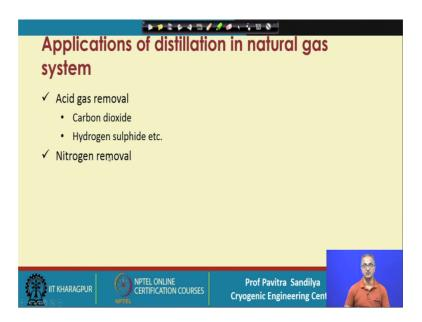
Now, coming to the applications of this distillation, in natural gas systems, we have basically go it for do for acid gas removal like carbon dioxide and hydrogen sulfide and nitrogen removal.
