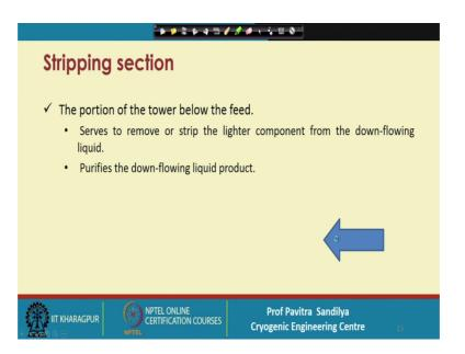
And it serves to remove the lighter component from the down flowing liquid; that means, the lighter components the liquid is coming down the whatever lighter components or high boil low boiling point components are there, they will be going more from the liquid phase to the vapor phase, thereby making the liquid richer in the high boiling point components.
