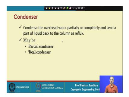
Next we have this top vapor is taken to a condenser and what are the condenser do this condenser each condenser condenses the overhead vapor partially or completely and it sense a something a liquid called reflux. So, this is the condenser and the condenser may be a partial condenser or may be a total condenser.
