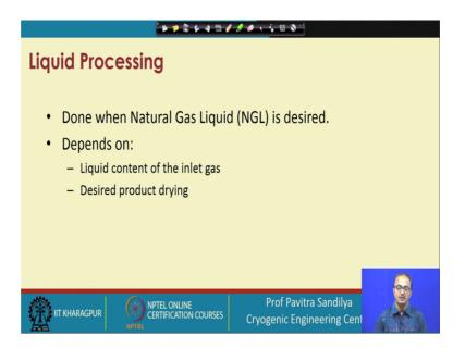
Next, we have liquid processing this liquid processing means that we are getting the natural gas liquid this is not LNG. LNG is basically the methane and methane and some other higher compounds, but NGL means some higher hydrocarbons other than methane they are also coming and there are also can be used at feedstocks for making other chemicals. So, they are also recovered as NGL and it depends on the liquid content of the inlet gas and the desired product drying.
