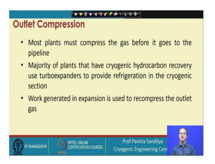
And then we need outlet compression this is that the gas which is produced need to be compressed when before it goes to the pipeline, to make it flow, generally, the natural gas which is obtained from the reservoir comes at a very high pressure. So, there we do not need to compress it much the natural pressure itself can make it drive make it flow through the pipelines, but on the outlet side after undergoing many processing the pressure comes down.
