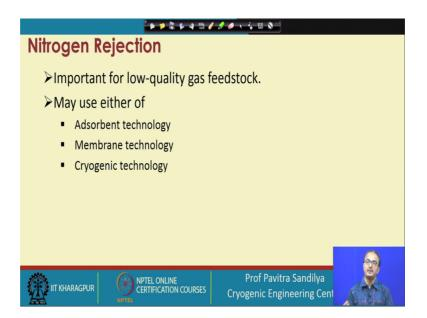
Next is nitrogen removal. Nitrogen is also very important and very significant amount of the natural gas is having nitrogen and so, nitrogen is an innovate gas as such as does not react with other components. But it reduces the calorific value and that is why it is important to remove the nitrogen and there are various technologies to remove the nitrogen. Some of them are like adsorption by which we mean that we use some kind of solids to remove the gas adsorption.
