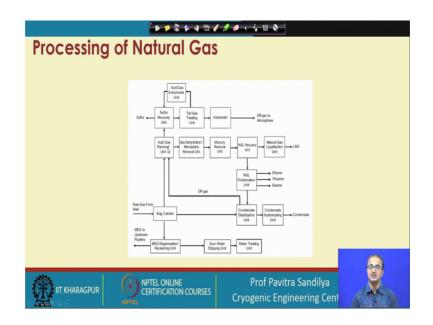
Now, with this; we see the various sources of natural gas, then we see the overall view of the processing of the natural gas because the raw gas which is coming to us that have to be processed to get rid of many impurities, before it can be consumed. So, in this particular figure we show the overview of the various types of processing first we see the raw natural gas is coming from here and then we are taking out various types of slurries and other slugs from this thing and there many things.
