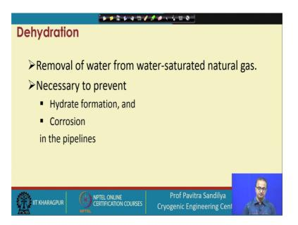
Now, we shall just quickly have a overview of the important processes in converting the raw natural gas into LNG. First, we come to dehydration means that removal of water and we know that the natural gas generally contains lots of water as it comes out from the sea and this water needs to be removed for that matter any impurities need to be removed so that we can get high calorific value of the natural gas.
