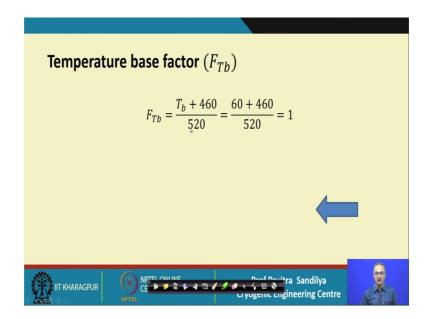
Next we come to the temperature base factor; in this case the temperature has to be in terms of the Rankine. So, here we put the Rankine pressure and temperature and we get it as 1; next we come to now just for recalling that temperature pressure are needed because they change the density of the gas and the density of the gas changes means that the volumetric flow rate for a given mass flow rate will also change that is why we apply the pressure and temperature correction factors.
