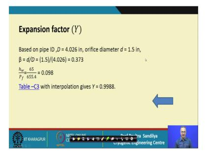
And lastly we have the expansion factor and this expansion factor is obtained from table C 3, but before that we have to find some parameter value like beta beta is the ratio of the orifice diameter to the inner diameter of the pipeline. With this we get the value of beta and then we find the value of this ratio h w by P f from the given data and we get this value.
