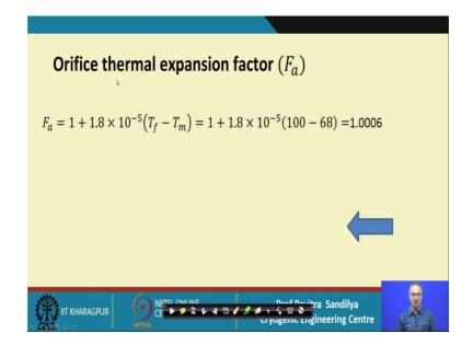
And then we have the orifice thermal expansion factor using this formula this is the fluid temperature 100 and this is the manometric this temperature that is 68 and with this we get the value of 1.0006.
