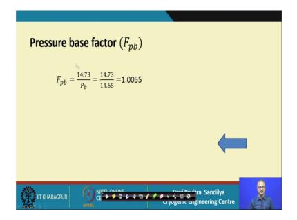
Next we come to the another correction factor that is the pressure base factor; here we are using this particular formula; please note that in this formula the pressure has to be in terms of psia. So, we are putting this pressure value here and we are getting this value of the pressure base factor.
