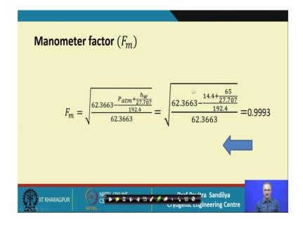
Next we go to this value of the manometer factor here we have the manometer factor with this particular formula it does not need any kind of charts, simply we put the atmospheric pressure the water column height and with this particular formula we get the manometer factor as 0.9993.
