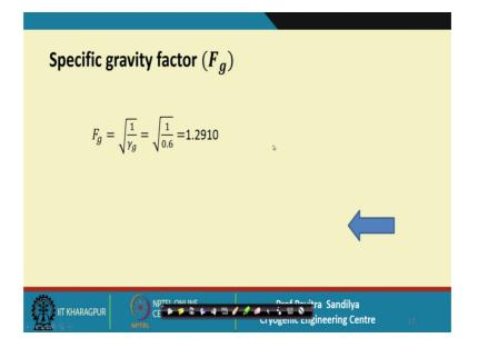
Next we come to the gravity factor; the gravity factor is taking care of the specific gravity of the gas which is given as 0.6 and this is the value.
