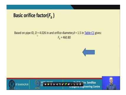
So, let us first look at this basic orifice factor and this basic orifice factor is based on the inner pipe diameter and the orifice diameter.
