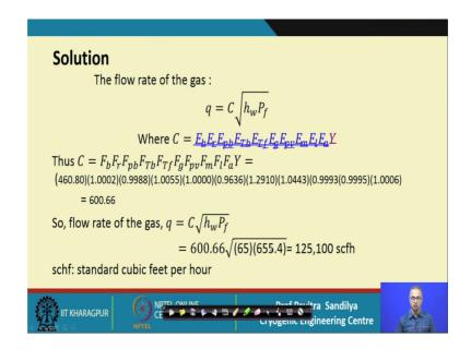
So, in this case it is specified that we have flange taps and if you recall we can see that how these taps were looking; that these taps were given in terms of the their distances from the flange. So, in case of flange taps the taps are just on the flanges.
