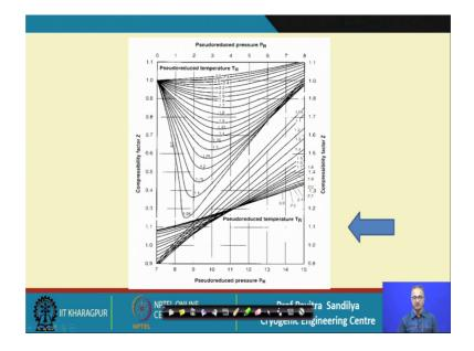
Here we have the P R that pseudo reduced pressure and on this here the reduced temperature and accordingly we can find out the value of the Z. So, knowing the P R and
