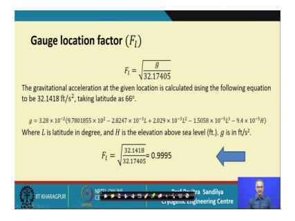
And next we have the gauge location factor this takes care of the gauge location depending on the latitude and the elevation from the sea level.
