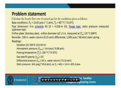
So, first let us take up a problem on the flow measurement here we are given that to calculate the hourly flow rate of natural gas for the given conditions. Here there are various conditions are given as we will find in the equation for the orifice meter which we saw earlier. First is the base condition here the things are given in fps units because the equations we learned they were having the fps units.
