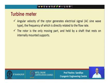
Here we see that angular velocity of the rotor generates some kind of electric signal that is AC signal which is related to the flow rate and the rotor is the only moving part here, and this is held by a shaft on an internally mount this support.
