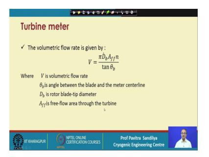
The volumetric flow rate through a turbine is given by this particular thing. In this case the V is the volumetric flow rate; theta b is the angle between the blade and the meter
