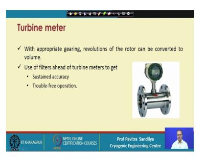
And with appropriate gearing arrangement, the rotation the revolution of the rotor can be converted to the volume of the fluid passing through the meter. Some kind of filters are filters to reduce the noise and to get better accuracy and trouble-free operation are used before the turbine meter. So, here we have shown a typical turbine meter which gives some reading in this particular recording device.
