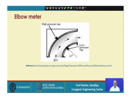
Elbow meter we know that it looks like this that here the flow takes place, and it goes through a curvature. And whenever it is a curvature effect, there will be some kind of a centrifugal force. And the centrifugal force will be changing along this diameter. Now, if
