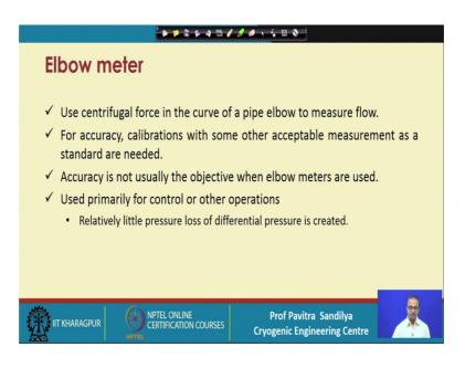
Next, we come to elbow meter. The elbow meter works on the basis of the centrifugal force.
