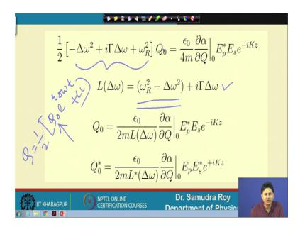
The delta omega thing I write this entire stuff as L function of delta omega to reduce or to make the calculation more compact. So, L of delta omega is omega R minus delta omega square plus i of gamma delta omega.
