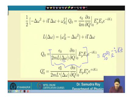
So, the amplitude part contain from here to here with the phase e to the power of say minus i kz. So, the complex amplitude Q 0 a is now in this particular form why this complex? Because E p E s may be complex and here L sitting here which is also complex. So, we can write the total Q 0 as epsilon 0 this, E p star E s and here in amplitude here in amplitude and phase form.
