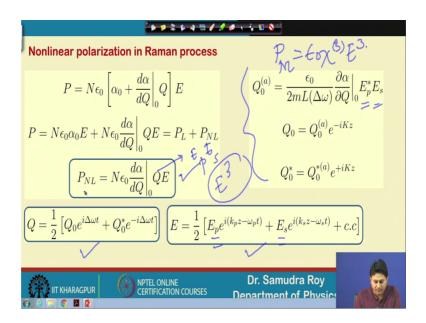
So, once we have Q 0 in our hand the next thing is to find out the non-linear polarization in Raman process that is the ultimate goal because non-linear polarization is something that we need to figure out.
