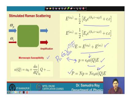
So, if I now try to understand these things in terms of mathematical treatment, then omega p omega s is launched. Omega p and omega s corresponds to the field frequency are the two frequencies corresponds to the field E p and E s which is the pump field and stoke field. In the plane wave form I can write the pump and stoke in this particular form, which we already used. Total field is omega p and omega s E omega p plus E omega s this is a total field.
