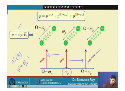
Well if I now try to understand that exactly what is going on and this is a pictorial figure for that, that as I mentioned this microscopic polarizability now vibrating three different frequencies. So, these 3 different frequencies give rise to three different waves and these three different waves if I write in the output if I try to find out what is the spectrum of this three different wave.
