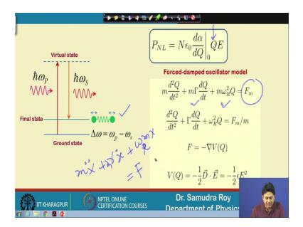
Next, next we need to find out what is the differential equation for the molecule. So, when the electric field is launched what happened the molecules goes from ground state to virtual state and returned back to some final state with a vibration and this vibration should have frequency. Delta omega which is the difference between omega p and omega s. S
