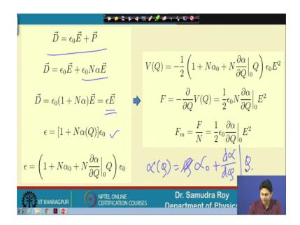
Well how to find out this. So, in this slide we will going to understand. So, total D is epsilon 0 E P we know, P here is the polarization we know this polarization can be represented in this way epsilon 0 N alpha E because alpha is a microscopic polarization everything. So, far we are doing in is in terms of microscopy polarization. So, d is epsilon 0 1 plus n alpha E and this is epsilon E. So, epsilon I can extract from this equation.
