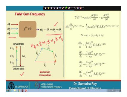
So, let us try to find out what we try to say here. In Four Wave Mixing, there are different kind of categories because the generation of the frequencies are large. So, this is a typical example of some frequency generation. So, what is happening here, I am launching 3 fields with frequency omega 1, omega 2 and omega 3 as shown in here. K 2 is not equal to 0; that means, we should have a non-linear interaction between these frequencies, this non-linear interaction will be of the order 3.
