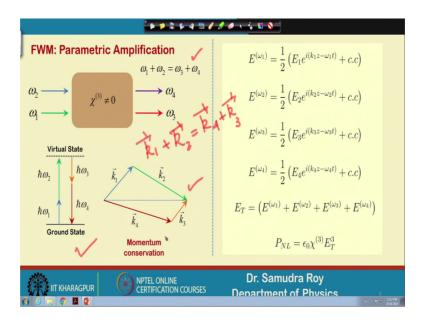
Now, we will go to the next thing which is Parametric Amplification. So, some frequency generation is one kind of Four Wave Mixing, but parametric amplification is quite interesting, where omega 1 and omega 2 are launched and we are getting omega 4 and omega 3 at the output. So we are launching two frequencies omega 1 and omega 2 and we are getting omega 3 and omega 4.
