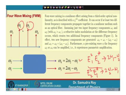
So, one combination maybe one combination maybe E 1 square E 2 star; so, E 1s it is. So, E 1 square E 2 star basically give raised to one frequency 2 of omega 1 minus omega 2 which is this one. So, this combination basically give raise to a frequency omega 3 and also another combination can be possible which is E 2 square E 1 star which give us 2 omega 2 minus omega 1. So, another frequency is there.
