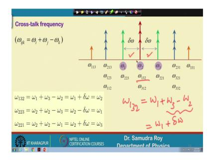
So, this is the matrix of the frequencies and now, we try to understand how this frequency are located. For example, let us start with omega 1 3 2 this frequency how this frequencies are generating? Omega 1 3 2 is essentially omega 1 plus omega 3 minus omega 2.
