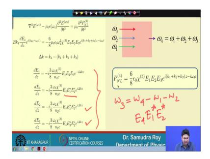
So, I now I have P non-linear term in our hand and if I manipulate the non-linear Schrodinger equation for E 4 term. So, it will be simply it will be simply this quantity. So, this is the non-linear Maxwell's equation that we have been using to generate the
