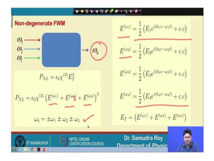
Once we have the idea of degenerate and non degenerate frequency. So, let us try to find out how mathematically we can understand that or how the treatment is done. So, for non non degenerate 4 wave mixing, which is a most general case omega 1, omega 2, omega 3 is launched and as a result I am generating omega 4.
