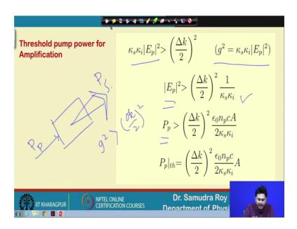
So, this threshold condition we can find out quite easily because g inside g we have the information of pump inside the g we have the information of the pump which is this.
