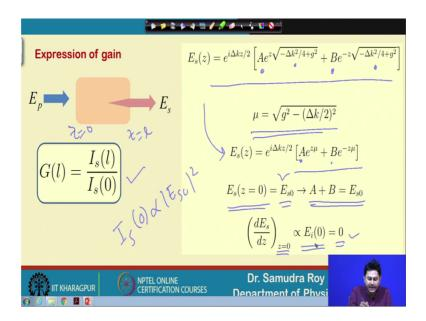
Well, after having the expression of this pump now, we try to find out what should be the expression of the gain that we are talking about. So, we are launching some kind of E p and generating E s. So, the gain means whatever the value we have at the initial point at z equal to 0, for the corresponding intensity or power.
