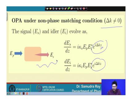
So, the condition that is imposed here is delta k not equal to 0. So, delta k not equal to 0 essentially means the phase matching the phase matching is absolute phase matching absent.
