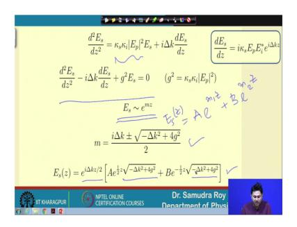
So, this is the expression that we have right now; this term is replaced by g square. So, this is the differential equation we have a standard second order differential equation having the first order differential term. So, when once when we have this kind of equation this is some sort of homogeneous equation we do not have any kind of source term here. So, the life is easy here.
