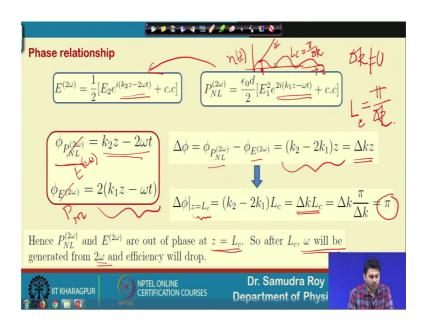
Now, the question is what is the phase relationship between so, in the previous curve we see that electric field is launched here and second harmonics is generating here. So, second harmonic basically is generating because P non-linear 2 omega is generating.
