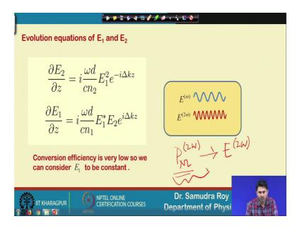
So, this is the reason why E 2 is generating. So, P non-linear 2 omega is a quantity which is important because this is the source term for second harmonic. So, now, the next thing is to understand what is the phase relationship between E 2, which is generated and the corresponding source term that is constantly feeding the energy to E 2; that means, P
