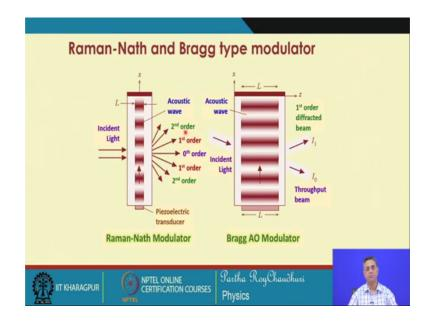
But, in the case of Raman-Nath, it could be a normal incidence and we will get a number of diffraction orders. So, let us recall this Raman-Nath type of diffraction, where the incident beam normally incident on this acoustic cell, Raman-Nath modulator cells. And there will be various orders 0th order, plus order, minus order, 1st order, 2nd order and so on this is the propagation of the acoustic wave. So, this gives a very clear picture and understanding about this.
