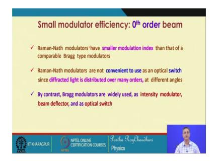
So, small modulator efficiency; the Raman-Nath modulators have smaller modulation index than that of the comparable Bragg type of modulator, Raman-Nath modulators are not convenient to use as an optical switch since the diffracted light is distributed over many orders and that too happens at different angles therefore, it is difficult to track all of them. By contrast, Bragg modulators are widely used for optical modulator, beam deflector and also optical switches.
