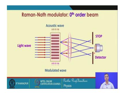
So, we can put the detector at the 0th order, and we stop all the higher orders. So, in the case of we just look at the variation in the intensity in the 0th order. So, this is how the light wave is incident, it passes through this modulator. You have a lens, which will collect the beams at various orders so, this here you will get the 0th order in front of which there will be a detector.
