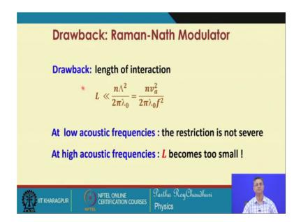
Therefore, the problem with this the drawback using the system that the length of interaction L comes from here at low acoustic frequencies, this restriction is not severe. But, at high acoustic frequencies L becomes very large.
