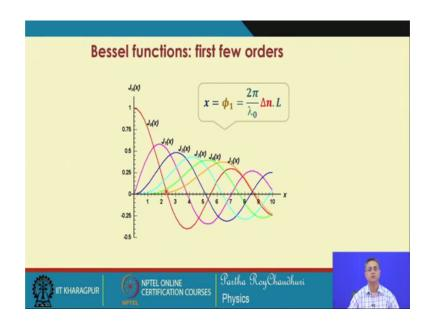
So, therefore, the various orders of Bessel function, we may recall that this is J 0, J 1, J 2 etcetera. So, they have different zero crossings and it is only the J 0, which is maximum at x equal to 0, in this case phi 1 equal to 0.
