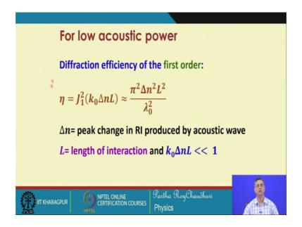
And this is for low acoustic power, we have also seen that. This diffraction efficiency can be simplified in this form pi square delta n square L square by lambda square. As a result, the peak change in the refractive index produced by the acoustic wave. This and this length of the interaction, therefore, this will be less than k 0 delta n and L.
