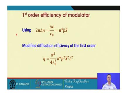
So, now again the one which we have used that n equal to n cube, n cube half n cube p into S. So, if I use that, so delta n will be equal to half n cube p into S will give you the diffraction efficiency in this form. Using this case for this case that is when the acoustic power is low and we have seen how we can approximate the diffraction efficiency as this.
