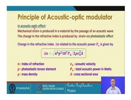
So, the basic principle let us remember that the mechanical strain, which is produced by the passage of an acoustic wave is to create a refractive index modulation, why this photoelastic effect. And the change in the refractive index, the peak change that is the maximum change the modulation depth delta n is related to the acoustic power by this.
