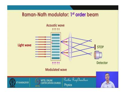
So, in this case, you look at the design of the modulator for the 1st order beam. You have this optical acousto-optic cell and the light beam is incident normally on this cell and various orders various diffraction orders. And now in this case you put a stop at the 0th order, but you put the detector at the 1st order. And take the signal out from this, which will give you the modulated signal the way this acoustic wave will be modulated.
