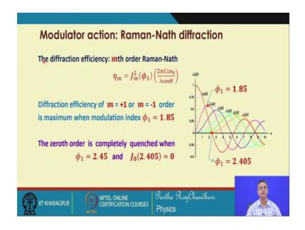
Therefore, the diffraction efficiency in the mth order will come from here J 1 square J J m square phi 1; phi 1 is phase, which will come from here. Now, the diffraction efficiency in the plus minus 1 order is maximum when the modulation index phi 1 is equal to 0, because that is the 0 of the Bessel function J 1. You can see this the this is the
