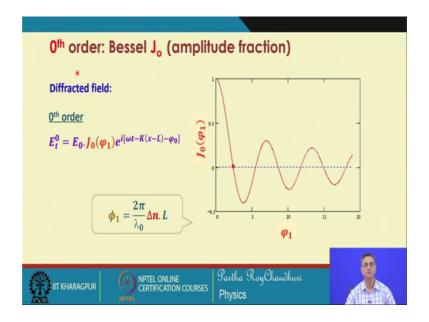
Now, look at this for the 0th order diffracted beam you have this 0 of the Bessel function, which corresponds to 2.4048, 2.4045 at this point. So, this is the flexible, this is the
