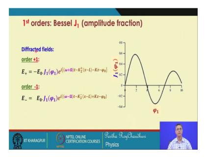
1st order first order Bessel function, if you look at this, you see this is the expression for the amplitude of the light electric field amplitude of the light, which is diffracted in the 1st order and this is the amplitude for the minus 1 order. And you can see that this amplitude, it becomes maximum at this point it becomes maximum at this point, you can see this amplitude becomes.
