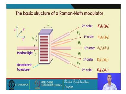
So, we will continue our discussion with this. So, the schematic of this Raman-Nath type of modulator is you have an incident beam, which is incident normally. And this is the beam width, you have this acoustic wave length capital lambda and the beams are diffracted this is the 0th order beam, plus 1 order, plus 2 order, minus 1 order, minus 2 order and so on and so forth.
