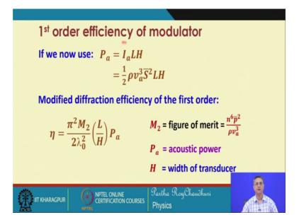
1st order efficiency of the modulator if we now use this relation, that is acoustic power and acoustic intensity relation, which will finally lead to this diffraction efficiency for the 1st order, we can write in this form. A very simple straight forward algebra and M 2 is the figure of merit, which is given by this. And I said this is common and the P a and H are defined as the acoustic power and this.
