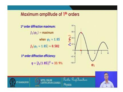
Therefore, starting from 0, so when you have phi 1 equal to 0, you have no light in the 1st order diffracted beam. But, when this phi 1 the phase change phi 1, which will be modulated as delta phi equal to phi 1 sin of omega t or sine of k z periodically along the length of the of the acoustic wave. So, this is the value of phi 1 when it is equal to 1.85 this value, you get that the maximum power in the 1st order diffracted beam. And that gives you the modulation starting from 0 up to this.
