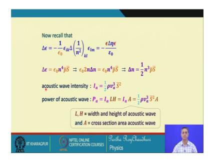
So, this is the basic principle that an acoustic wave propagates. There is a periodic change, there is a modulation of the refractive indices, which is travelling with the velocity of the acoustic wave. And now that optical beam will get diffracted depending on the acoustic wave characteristics, the beam can be optical beam can be modulated.
