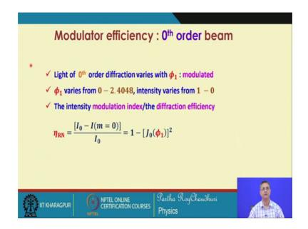
And the diffraction efficiency in this case will be equal to m equal to 0. So, I 0 and for the 0th order this is the incident beam and the intensity of the 0th order beam. So, from here, we can calculate the diffraction efficiency. The intensity modulation index or the diffraction efficiency is given by this equation, which is very straightforward.
