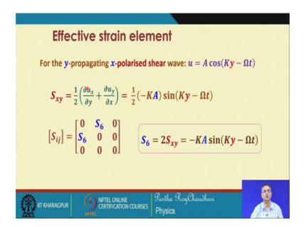
So, it is u x with y that change is non 0 del u x del y this quantity is non-zero, so that gives you this S x y is equal to this. And in the same similar way we can write that S 6 which will occupy these two up diagonal positions, and that gives you this S 6 equal to twice S x y. And this quantity this we have seen earlier also in the same way.
