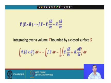
So, let us look at this; del dot E cross H minus B equal to minus j E minus E dot del d del t minus H dot del t. We have just rearranged this equation in a fashion that, we have taken this quantity and this quantity together which is a like and this quantity we have placed separately. The mission the reason is very clear that we want to look at these terms these two terms put together and also this term J dot E d v.
