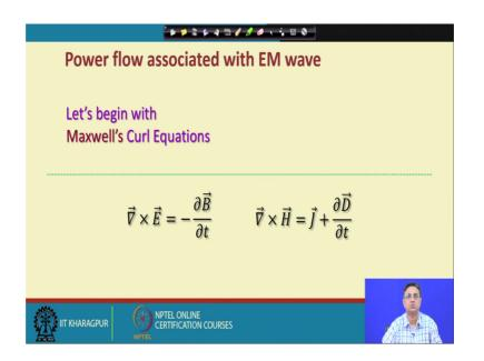
So, let us begin with the Maxwell's curl equations, we have these two famous curls equations that del cross E equal to minus del B del t and del cross H equal to j plus del D del t where B is the magnetic field and D is the displacement current j is the induction current.
