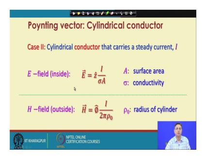
Now, we will consider another interesting case where we will see the Poynting vector through a cylindrical conductor that carries a steady current, I. Now the electric field inside this conductor is given by this E equal to z cap I by sigma into A, this is because this Ohms law if you write J into sigma is equal to E. So, sigma into E is equal to z into J.
