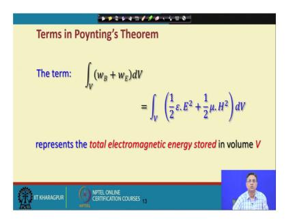
So, let us let us look at this term that that the energy density some of the energy density is for the magnetic field and for the electric field is equal to this just now we have seen. But because this is the total energy density with the electric field and magnetic field, so this quantity actually represents the total electromagnetic energy stored in the volume V.
