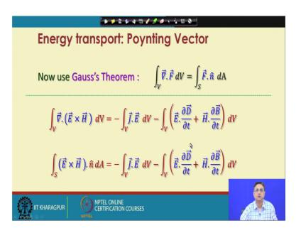
Now, look at these two terms we will use Gauss's theorem to see what is meant by this quantity del dot E cross E E cross H. So, Gauss's theorem states that it relates the volume integral to a surface integral for a vector field H the divergence of this vector field over is a over a certain volume is equal to the closed surface integral of the vector field.
