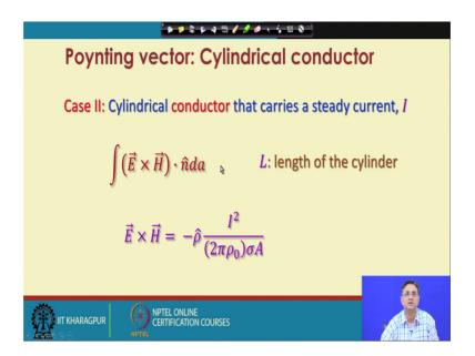
So, let us see that for the cylindrical conductor that carries a current I, we can write the Poynting vector in this way E cross H dot n d a where we consider a certain length L of the cylinder.
