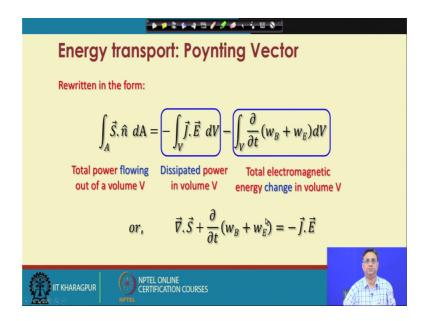
Now, again rewriting this equation in this form, this left hand side that is the term which contains the Poynting vector represents the total power flowing out of the volume V which is equal to the power in the volume dissipated power in the volume and also the total electromagnetic energy change in the volume. This is just now I have mentioned
