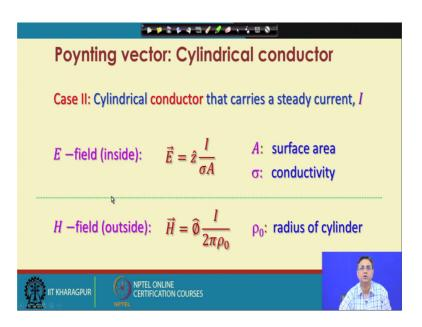
So, E cross H if we put together, this E cross H and take the cross product of these two quantities, then we can represent that E cross H equal to minus rho cap unit vector of rho that is the radius vector direction by into I square by twice pi rho sigma into A.
