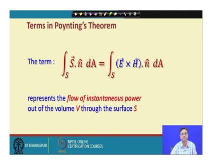
And if you look at this term that is S dot n d A which is equal to this, this actually represents the instantaneous power flow of instant instantaneous power instantaneous power out of the volume V through the surface S.
