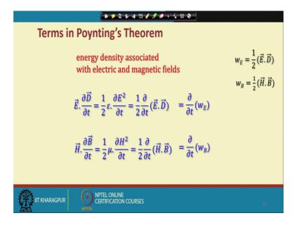
So, if we use definition of the of the electric and magnetic field energy density, then we can write that E dot del D del t which is equal to half of epsilon is replacing this D that is D equal to E into epsilon. So, half epsilon into del E square del t which can be rewritten
