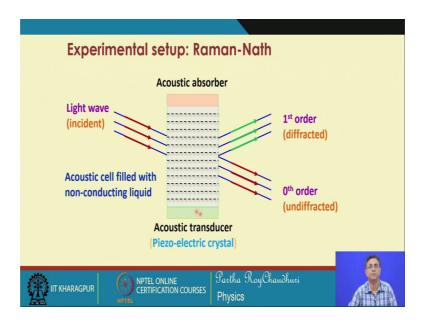
So, the basic experimental setup for this a Raman-Nath type of diffraction, you have a light which is incident here and this is the acousto-optic cell you have a transducer acousto-optic piezo crystal which is attach to this and we have some liquid which is non-conducting non polar liquid and this liquid fills and it behaves as the medium where the periodic refractive index will be generated.
