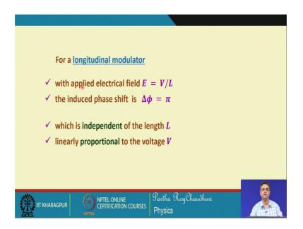
So, for a longitudinal modulation we see that the applied electric field e equal to V by L the induced phase shift del phi equal to pi and this is you can see that induced phase shift which is independent of the length of the modulator crystal. But it depends on the applied voltage depends on the applied voltage a phase shift is proportional to V, but it does not depend on the length of the crystal.
