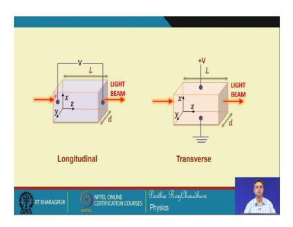
So, this is the configuration for a longitudinal mode of operation you can see this is your x, y and z you apply a voltage along the direction of propagation of the light beam. But in this case the voltage that is the electric field that we apply across the crystal a direction which is perpendicular to the direction of propagation of the light.
