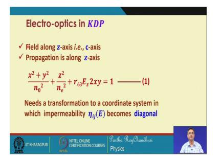
Now, if we assume that the electric field is along z-axis that is the C-axis of the crystal and the light is also propagating along z-axis that is this longitudinal mode of operation you have light which is travelling along x-axis and electric field is also applied along the z-axis.
