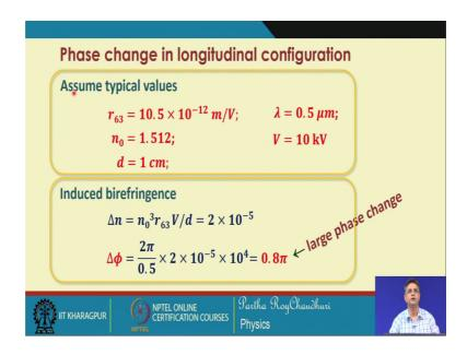
So, let us assume this typical values for r 63 which is 10 point that is at this wave length and V equal to let us suppose that it is 10 kilo volt if we apply this much have voltage
