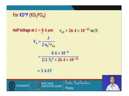
Half voltage for this KD star P dihydrogen phosphate this the coefficient is now more and as a result the half voltage reduces to 3.4 kilovolt which is as good as one-third times less than the half voltage of this one that is for the KDP crystal. (Refer Slide Time: 21:32)
