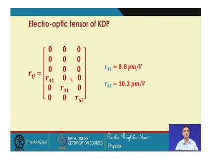
So, when you and the electro-optic coefficient that values we have already mentioned that r 41 is equal to 8.8 picometer per volt whereas, r 63 is so these two are the same value and this is different. And now these values will make the system different depending on the orientation of the electric field that is applied to the crystal.
