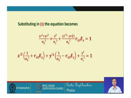
So, if we substitute this into this equation then we can we write this equation in this form, and then this equation becomes of this form x prime square 1 by n naught square plus. So, this is the additional quantity, additional term which has come along with 1 by n 0 square and similarly for the y square term is now associated with these two components. So, these are the new refractive indices in the principal axes system.
