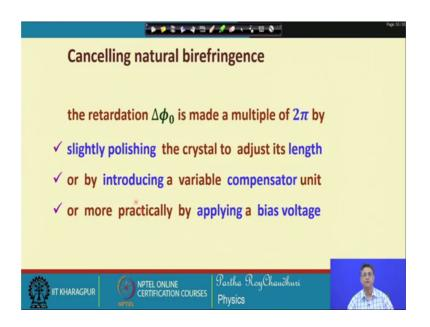
Now, so this canceling this, this is one important requirement that just to make this is the birefringence is just proportional to the applied voltage we need to cancel this natural birefringence which can be done by optical biasing or by applying a bias voltage. So, this retardation delta phi is made a multiple of twice pi, which can be done by slightly polishing the crystal to adjust its length. Because it is length dependent natural birefringence is length dependent k 0 delta n x y into l.
