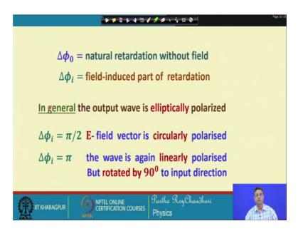
In general the output wave is elliptically polarized. But if you if you are induced birefringence say size that which is an electric field dependent property voltage dependent property is equal to pi by 2,then the electric field vector is circularly polarized that the output, but if it is pi then it will be linearly polarized.
