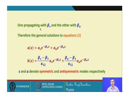
So, one of these 2 waves of the total system the composite system is propagating with a propagation constant beta s, and the other one is with the propagation constant beta a.
