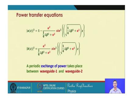
So, we write this equation in this form a z square and b z square. You can see that there is a the periodic exchange of power between the 2 waveguide, that is the periodicity will be twice pi is k twice pi by lambda this quantity.
