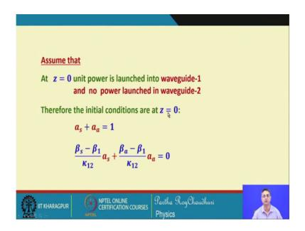
Now we have seen that if these 2 waveguides are identical and if I substitute this beta s and beta a by beta 0 plus k, and beta 0 minus k back into the this equation, into this equation, then we can write this expression for the a z and b z in this form, it requires a simple algebra calculation manipulation.
