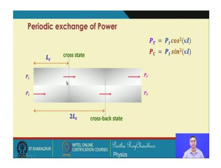
So, we have a visual favor of how this coupling takes place we have an input power in the waveguide 1. And it goes to waveguide 2 and then it again comes back to waveguide 1 and again goes to. So, in this wave the periodic exchanger power takes place back and forth between the 2 waveguide. This state is called cross state because we have entire curve which 2, the second waveguide this is cross back state where the power is restored back into the first waveguide.
