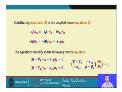
So, if I now substitute this assumption that there is a wave of that total system, and we substitute this wave back into the wave equation the couple mode equation then we can write this couple mode equation in this form. So, we get from the couple mode equation i beta (Refer Time: 14:40) del a del z will be give i beta and this was already i beta 1.
