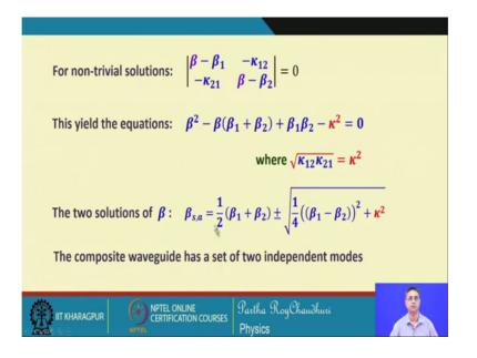
Which will give you an equation quadratic equation of beta square because you are looking for a beta, we have assume that there is a beta there is a total wave for the composite system, which is propagating with a phase constant with a propagation constant beta. And we are looking for this beta in terms of the amplitudes and propagation constant of the individual waveguide.
