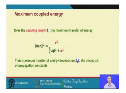
So, over the coupling length the maximum transfer of energy that is b z square will be equal to this for non-identical system, but if they are identical delta beta will be 0. So, this is equal to 1. So, that is maximum transfer of energy will take place from a z square and a z square at that moment will become equal to 0 and this will become equal to 1.
