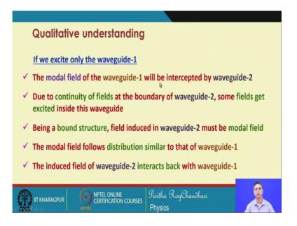
In that case, if we assume that we have exited one of the waveguide, let us suppose these waveguide will learnt field optical wave into this waveguide, then the modal field of the optical waveguide 1 will be intercepted by the waveguide 2.
