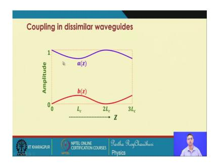
This we can so with a plot computed the plot of the amplitude transfer for waveguide a this is how it varies there is a small change because of the interaction. And in waveguide only a small part of the wave is coupled over the introduction. So, this is the coupling length over reach the maximum transfer of power takes place. This is the cross back state when again the power goes back into the first waveguide and so on.
