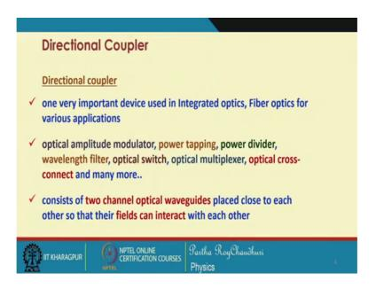
So, this is one very important device used in integrated optic, fiber optic a very useful component we will look at how this directional coupler are have include almost every part of the communication system and also a very useful device for sensor. Optical sensors, then optical many of the devices are like know very important in the in terms of this optical amplitude modulator, power tapping then power divider spliter, combiner,
