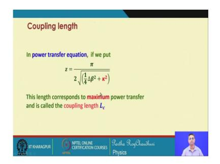
So, here if we put that z equal to pi by 2, and under root of this quantity. At this distance the length of the interaction between the 2 waves between the 2 waveguides, you can see if you put the value of z into that into that equation; that the length corresponds to maximum power transfer because this will give a sin function equal to 1 and cos function will become equal to 0. And is this length will be called the coupling length.
