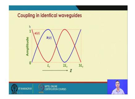
And then we can repeat this power variation in the 2 wave guide, where you can see that there has been a complete transfer of power; taken place between the 2 waveguide and this is the L c, the coupling length and you can also define the length overreach the power in the 2 waveguides are exactly 50 50. And that is what you call a 3 d B directional coupler, who will see some interesting applications of this 3 d b coupler in the following sections.
