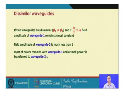
It is it is not 100 percent the field amplitude of wave guide 2 is much less than 1.
