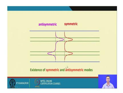
So, this beta s that is symmetric wave will have filled profile like this. You know this is the even mode and this will be antisymmetric which we call the odd mode.
