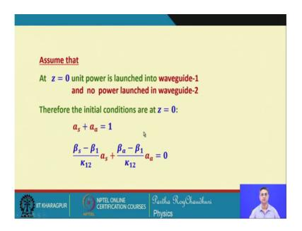
And we can assume that we can put the boundary condition, that have z equal to 0, if we at z equal to 0. If we launch unit power into one of the waveguide, I just launch unit power into one of the wave guide then these 2 amplitudes will be added up because the phase difference is 0 at z equal to 0, both of them will have z equal to 0 phase difference between them is 0. So, they will be added up and these 2 we will be cancelling each other.
