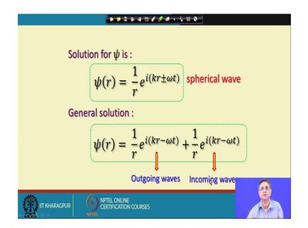
But we started with psi. So, to get back with a with an equation of psi we should write psi of r equal to 1 by r e to the power of. So, again will end up with the spherical wave and the general solution of this wave is psi of r 1 by r e to the power of i k r minus omega t plus e to the power of this should be plus. So, this is spherically outgoing waves and if you put a plus here it should be spherically incoming wave. (Refer Slide Time: 22:28)
