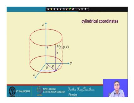
So, look at this cylindrical coordinates if I have my source sitting here, then on the surface of the cylinder the phases will be constant. The representation is this is the azimuth phi, this distance this is rho and the height is z is a usual notation for cylindrical coordinate system.
