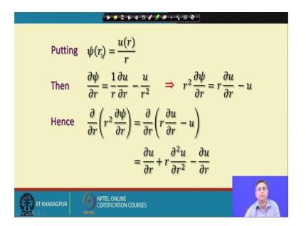
So, in this case we put there is one step that let us put psi of r equal to u of r by r. So, the equation del psi del r now becomes 1 by r del u del r minus u by r square. Just del del r if
