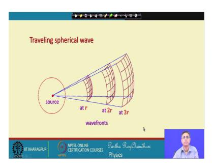
A traveling spherical waves you have a source, if you move radially outwards then they will form the wave front, which are the surface of the spheres. So, at a distance r the phases will be constant, at a distance 2 r the phases are constant and so on.
