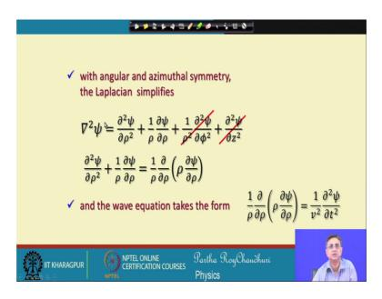
With angular and azimuthal symmetry, that is if I assume that it is independent of the azimuthal symmetry, we can write this equation only as a function of rho and the wave equation takes the form of this. Because you can remove these two terms because of the independent azimuthal symmetry the solutions of this wave equation.
