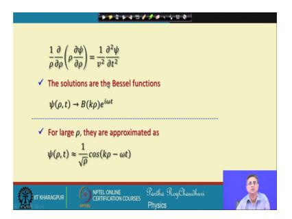
The solutions of this equation are well known Bessel functions and can be represented by this where this Bessel function has the argument of this propagation constant, and the radial coordinate rho times the e to the power of i omega t. For large distances rho this cylindrical waves are approximated as psi of rho t is equal to this.
