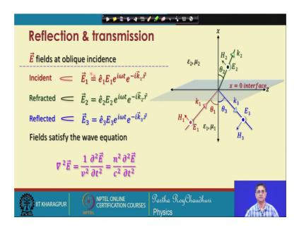
Now, E fields at oblique incidence we have this electric fields and each of them and also the magnetic field components will satisfy the wave equation. This we have seen earlier. Now, V square we can replace by n square by c square, where n square is the refractive index at the medium involved.
