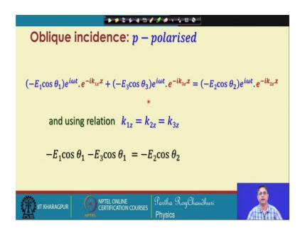
Therefore, and also we will use the relation k 1 z, k 2 z and k 3 z all of them are equal they are the z component of the tangential component of the propagation vector. So, k 1 z, k 3 z, k 2 z all of them are equal.
