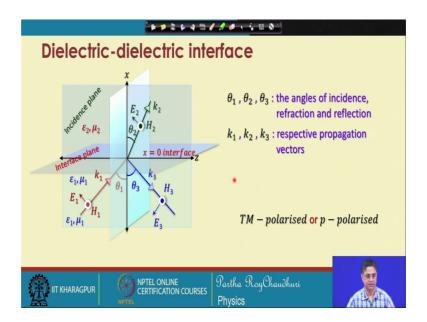
But, we also have to define the angles of incidence and angle of reflection and angle of transmission that is refraction as theta 1, theta 2 and theta 3. k 1, k 2 and k 3 these are the propagation vectors along the incidence direction, refracted direction and along the reflected direction. So, with this configuration the wave that we will discuss is the TM-polarised or p-polarised waves.
