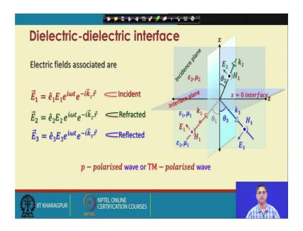
So, initially we will look at the properties of the medium in terms of the reflected and transmitted rays. Let us consider the electric fields plane wave fields associated with the
