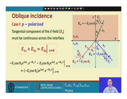
Now, let us consider few example cases. First is the in the case of p-polarised wave that is the present configuration that we have undertaken, the boundary conditions are the tangential component of the electric field must be continuous across the interface. The tangential component that is that is this component, this component and this component the tangential components tangential with respect to the interface they must be continuous.
