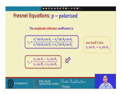
So, amplitude reflection coefficient we can even write in some modified form or reduced form rather we can say that r p is equal to this in terms of the refractive indices. But, now n 1 sin theta 1 is by the Snell's law we have just now seen that n 1 sin theta 1 for the first medium this is the angle sin of the angle with the refractive index is equal to n 2 sin theta 2 for the sin second medium.
