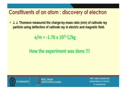
So, J.J Thomson measured the charge by mass ratio of cathode ray particle using deflection of cathode ray in electric and magnetic field. And he found the specific charge that is e by m equal to minus 1.76 into 10 to the power 11 coulomb per kg.
