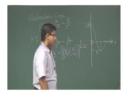
So, this is the equilibrium distance between atoms in a solid and that equilibrium distance depends on the on the atoms a b m dash n dash, these are the constant characteristic constants for atom and we have plotted earlier. I think I have to, so y axis is potential energy and x axis is basically r. So, if we think that one atom is here and another atom moving towards this atom.
