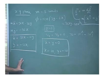
So, what do we get we get 2 equations of the form mx double dot will be equal to 96 x minus 36 y and m y double dot is equal to minus 36 x. Now recall that m is equal to 3. So, we put that and essentially we reduce this equations to x double dot is equal to 32 x minus 12 y y double dot is equal to minus 12 x. So, these are the sets of equations.
