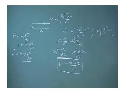
So, when we solve this problem; let us assume this is our fixed point, we said this as our origin o and here let us say this is the instantaneous position of this particle at a distance x from this fixed point. So, the velocity v at this point is given as some constant mu times root over x square; sorry; a square minus x square; a square minus x square by x square.
