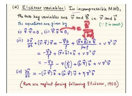
So, if you remember that the incompressible MHD, for example, the key variables are simply v and B, because  $\rho$  is a constant the fluid density is constant. So, simply we can write the whole thing in terms of v and B. Of course, we have pressure I mean we have a pressure like variable, but we also know from our previous discussion that finally pressure can be solved in terms of velocity, and finally, the message is that in order to construct a dynamical theory we simply need only v and b.
