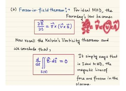
So, any vector field **A** if it satisfies evolution equation like this  $\frac{\partial \vec{A}}{\partial t} = \vec{\nabla} \times (\vec{v} \times \vec{A})$ , where **v** is the fluid velocity.
