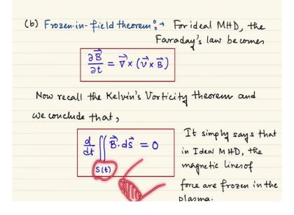
That is why  $\frac{d}{dt} \iint \vec{A} \cdot d\vec{s} = 0$ , where we are just talking about the any surface which is made by the fluid elements and moves with the fluid. So, of course, if it is made by the fluid element so, it is a real surface which is containing the fluid elements.
