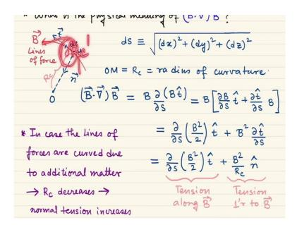
In the case, if you can see that you have the magnetic lines of force which are getting much more curved due to some additional matter or some increase in the magnetic field intensity and when it is getting curved then it's radius of curvature decreases. So, radius of curvature now decreases this is now  $R'_c$ .
