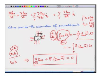
Since, this is a volume element, and space and time they are not seeing each other. So, basically by the Leibniz rule, the differentiation w.r.t time actually can enter inside the integration as a partial differentiation. So,
