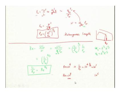
So, given viscosity and injection rate I can get  $l_{\nu}$ . Now, is one funny thing in that this is funny formula, right because your dissipation length scale Kolmogorov depends on injection rate, is not mean free path length this tells you that. The mean free path length cannot depend on how I how much energy I am injecting. If I inject more energy, then I can push my  $l_{\nu}$  smaller value?
