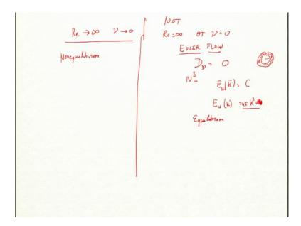
So, we assume that Re tends to 0, it tends to infinity or viscosity tends to 0, but it is not Re equal to infinity or  $\nu$  equal to 0. This is called Euler flow, if viscosity is 0 is called Euler flow and turbulence is, viscosity tending to 0, I need a cascade, viscosity is not there then there is no dissipation of energy. If there is no dissipation there is no flux and nothing.
