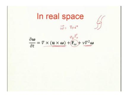
So, real space, vorticity is curl of  $\mathbf{u}$  is a vector,  $\boldsymbol{\omega} = \nabla \times \boldsymbol{u}$ , we are working with 3D. we will come to 2D later, but vorticity in it is like a vortex tube. So, this vortex and vortex tubes.
