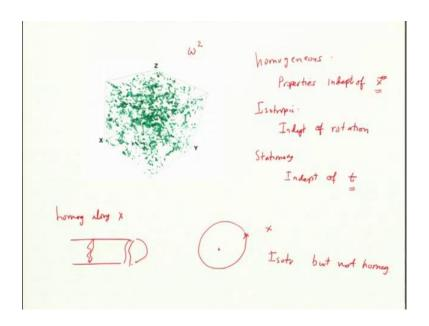
For homogeneity and isotropy of turbulence, this is from stimulation on a periodic box, which we did in our lab. So, this is verticity squared, it is a scalar quantity is magnitude a different positions are shown. Now, we can see that like is not coming from point source sitting in the middle. This is homogeneous in the sense no position is preferred.
