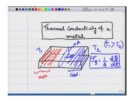
So, what is thermal conductivity? Thermal conductivity is related to having a metal which has a hot and cold end, let us take a piece of metal and you have a hot end and a cold end. And let us say one end of it is hot, this is hot end and you have another end which is cold.
