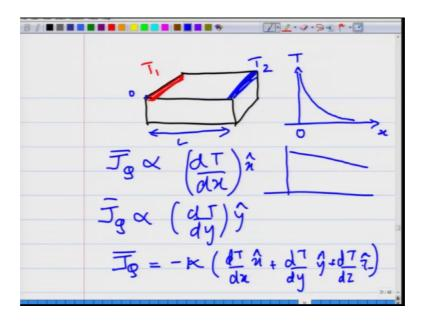
Namely, if you have this sample and this is your hot end and this is your cold end, ok. This is that temperature T 1 which is higher and this is at temperature T 2. Then, the amount of heat current that is going to flow will depend on the gradient, namely this temperature difference is maintained over how much distance L, ok. So, the amount of heat current which will flow will be proportional to the gradient.
